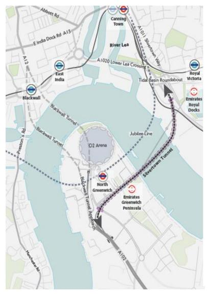
The Silvertown Tunnel would be a new twin-bore, dual carriageway road tunnel beneath the River Thames linking the A102 on the Greenwich Peninsula to the Tidal Basin Roundabout in the Royal Docks area.
