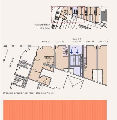
Figure 3: Plans of proposed solution to achieving Step Free Access to Thurloe Street and the South Kensington pedestrian subway
