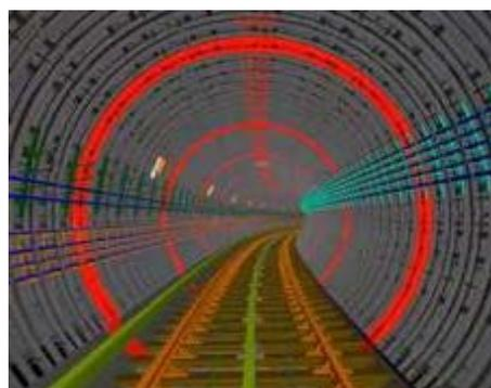
concrete rings in the southbound Jubilee line tunnel were deteriorating. It was clear we needed a long term solution. In 2010 partial ring replacement using spheroidal graphite iron segments was successfully trialled at Charing Cross in a disused section of the Jubilee line constructed in the same way as the tunnel between Baker Street and Bond Street.
