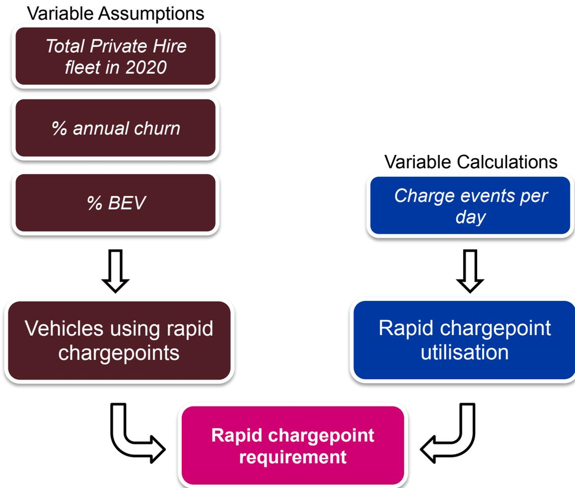
Figure 3 - Key variables considered to calculate rapid chargepoint requirements.
