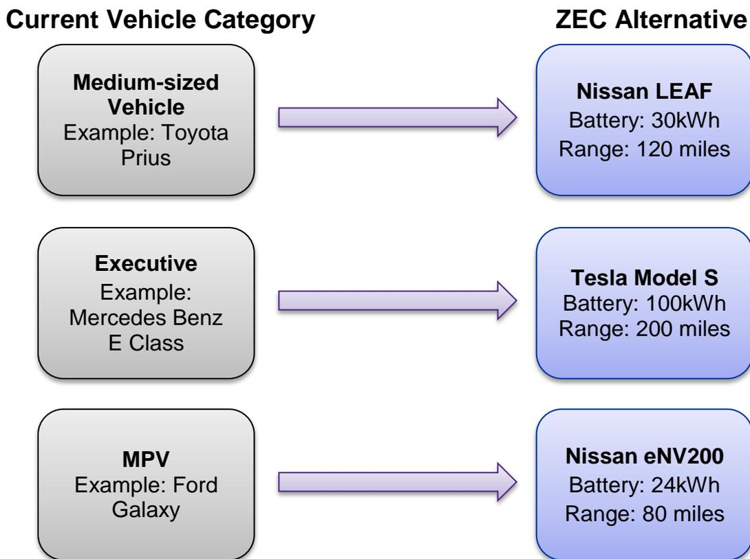
Figure 2 - Vehicle categories and selected ZEC alternatives' specifications. These specifications were used to inform the telematics analysis.
