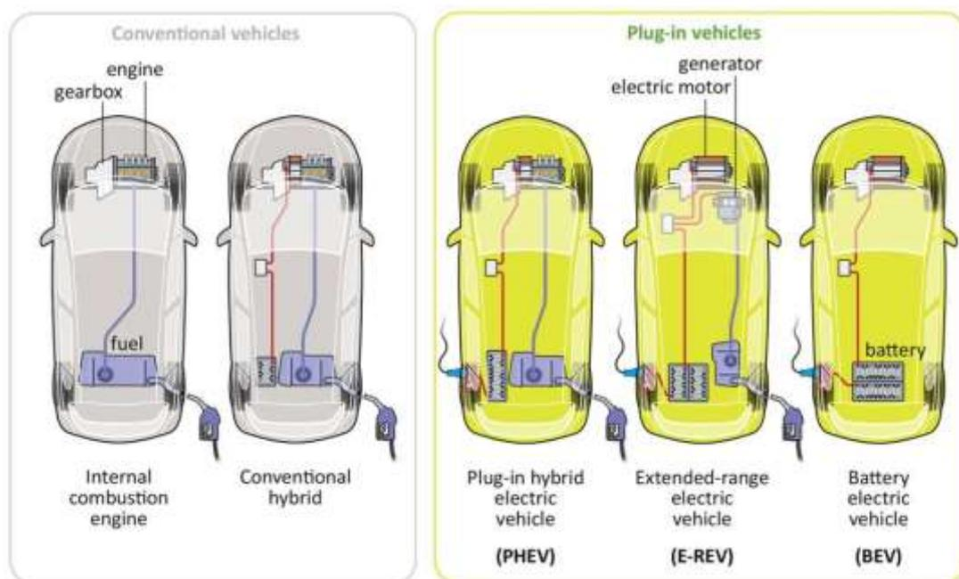
Figure 5 - Drivetrain technologies. Source: The Office for Low Emission Vehicles.
