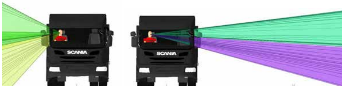
Figure 496. Frontal views of the off side and near side door window projections for the Scania N3 LEC
