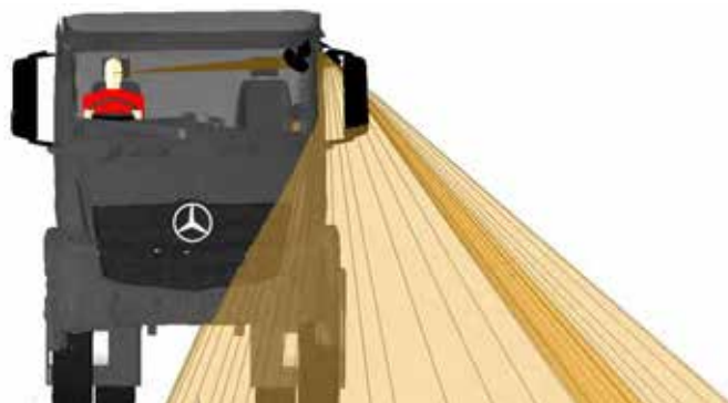
Figure 306. A front view of the Class V mirror projection for the Mercedes Arocs N3G
