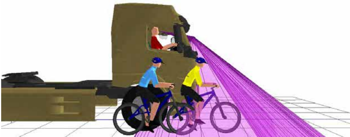
Figure 545. 3D view showing that the front (yellow) cyclist positioned to the offside of the vehicle is visible in the projection of the Class VI
