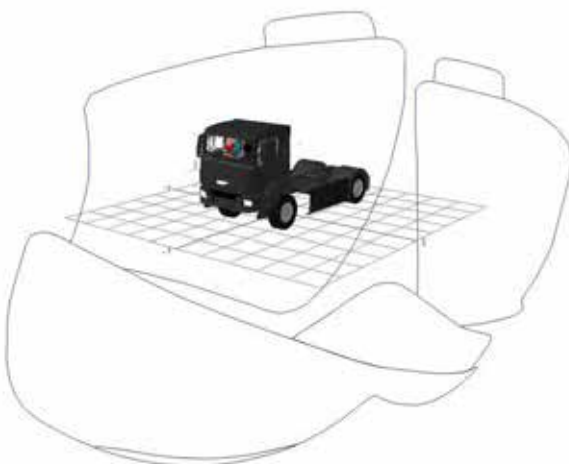
Figure 865. Combined indirect FOV area projection for the MAN TGS N3 / N3G
