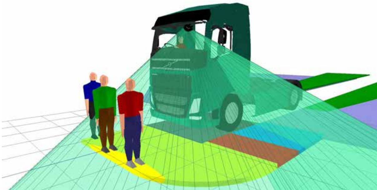
Figure 752. 3D volumetric projection showing the visibility of pedestrian VRUs to the front of a vehicle with a 5 th %ile UK female driver using the Class VI mirror adjusted for a 95 th %ile UK male
