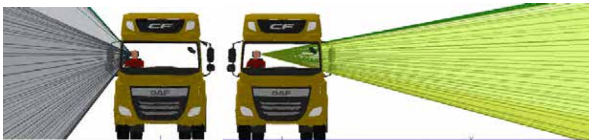
Figure 49. Frontal views of the off side and near side door window projections for the DAF CF N3
