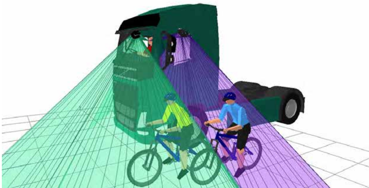
Figure 617. 3D view showing that both cyclists positioned to the nearside of the vehicle are visible in the projection of the Class V and / or Class VI mirrors
