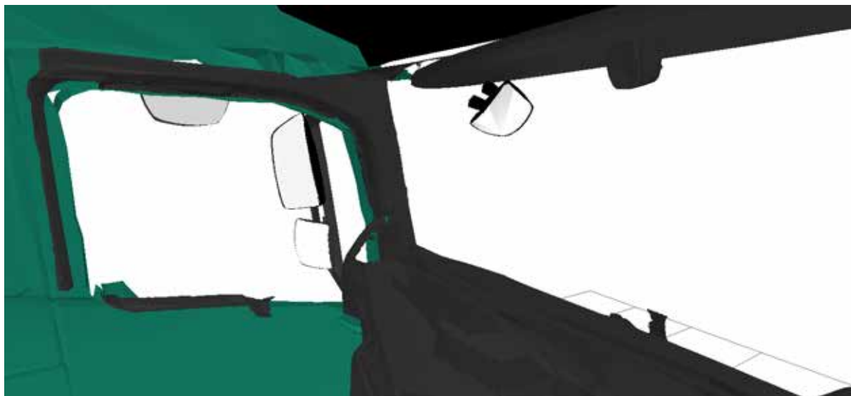
Figure 615. The view from the driver's eyes clearly shows the two cyclists are hidden from view.
