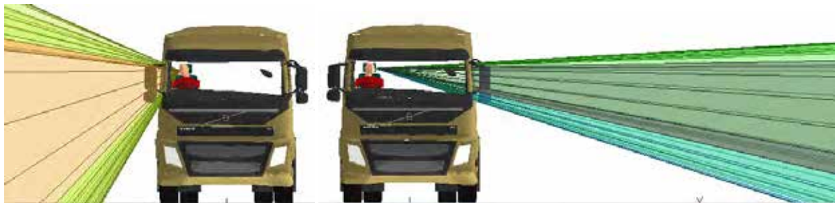
Figure 528. Frontal views of the off side and near side door window projections for the Volvo FM N3
