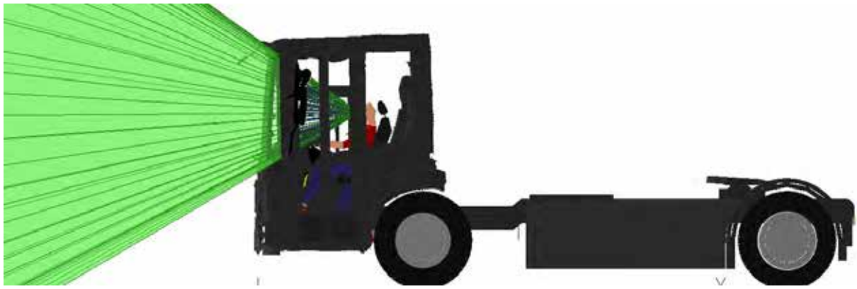
Figure 367. A side view of the windscreen aperture projection for the Mercedes Econic LEC
