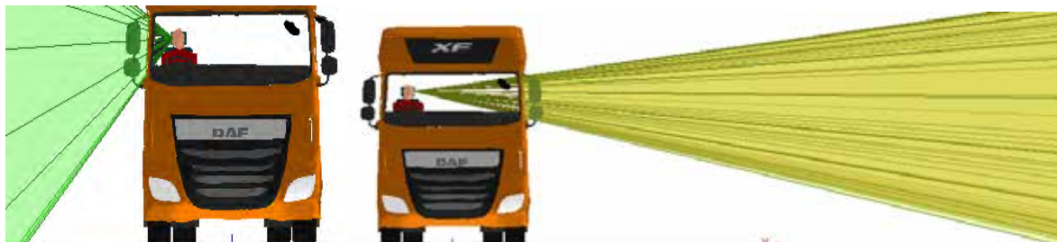
Figure 113. Frontal views of the off side and near side door window projections for the DAF XF N3
