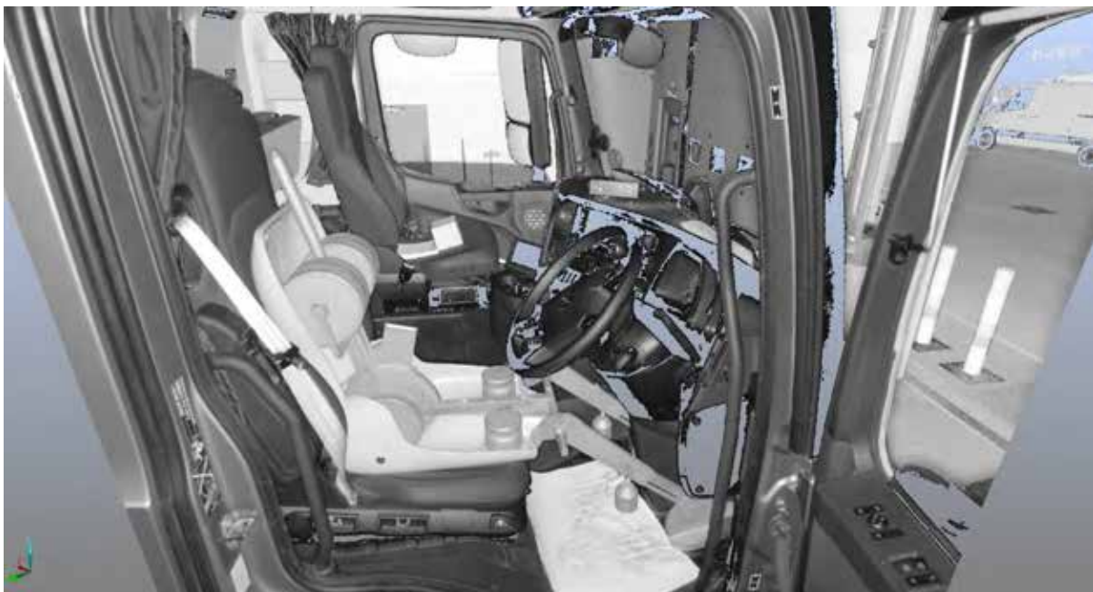
Figure 2. An example FARO Photon 120 scan of the interior of a vehicle
