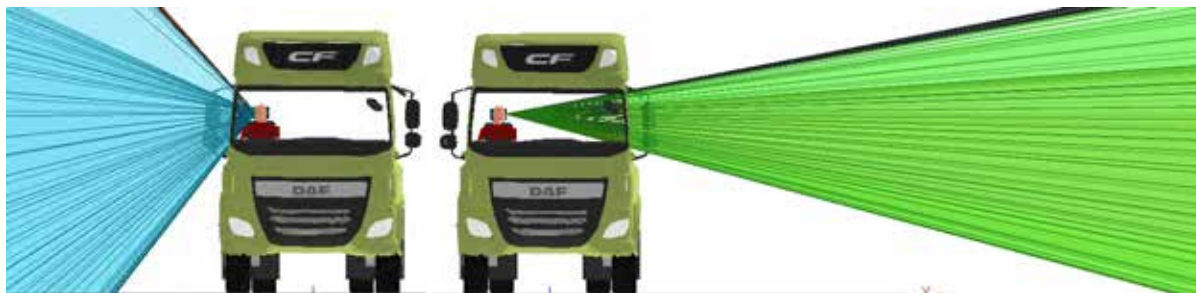
Figure 81. Frontal views of the off side and near side door window projections for the DAF CF N3G
