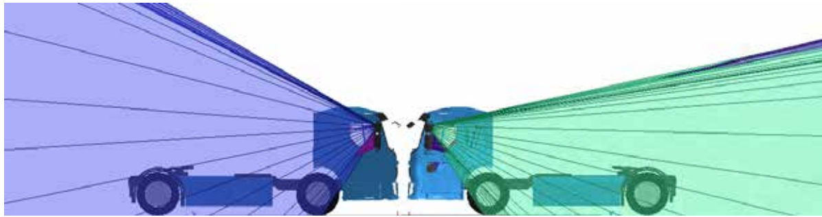
Figure 628. Side views of the combined Class II and Class IV mirror projections for the Volvo FE N3 LEC
