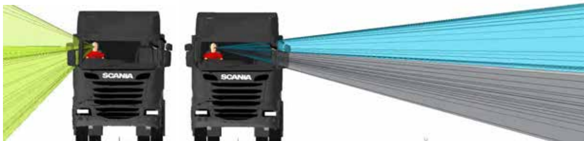
Figure 464. Frontal views of the off side and near side door window projections for the Scania R N3
