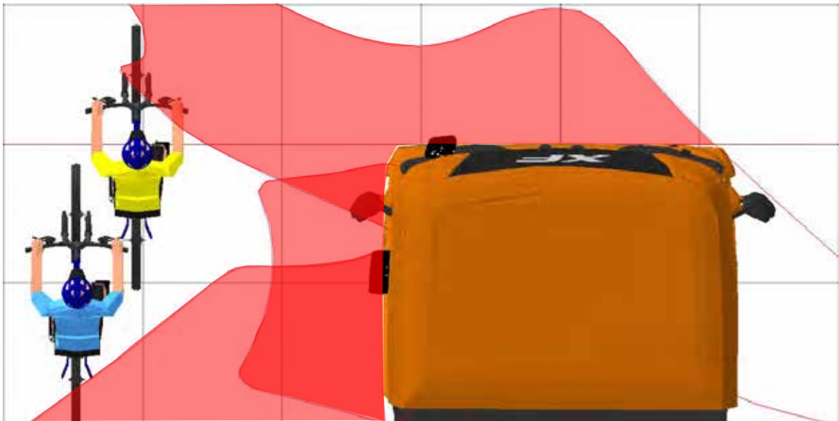
Figure 136. A plan view of the two human models that represent a cyclist moving up the inside of the vehicle and the projection of the Class IV, Class V and Class VI mirrors at a height that equals the stature of a 50th%ile UK male cyclist
