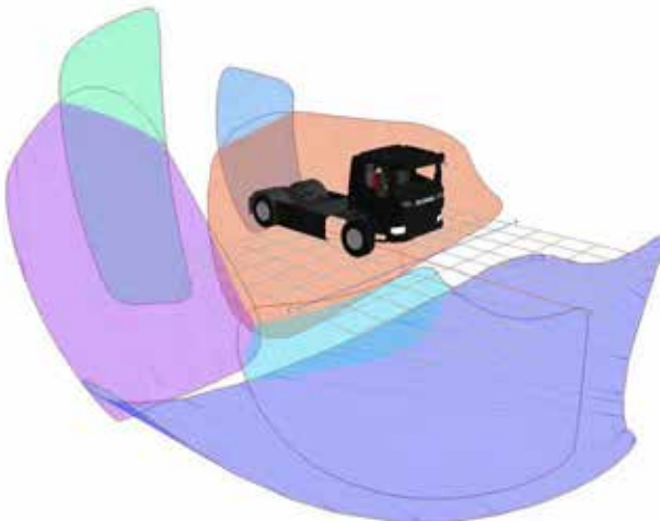
Figure 685. Indirect FOV area projection for the Scania P N3 / N3G
