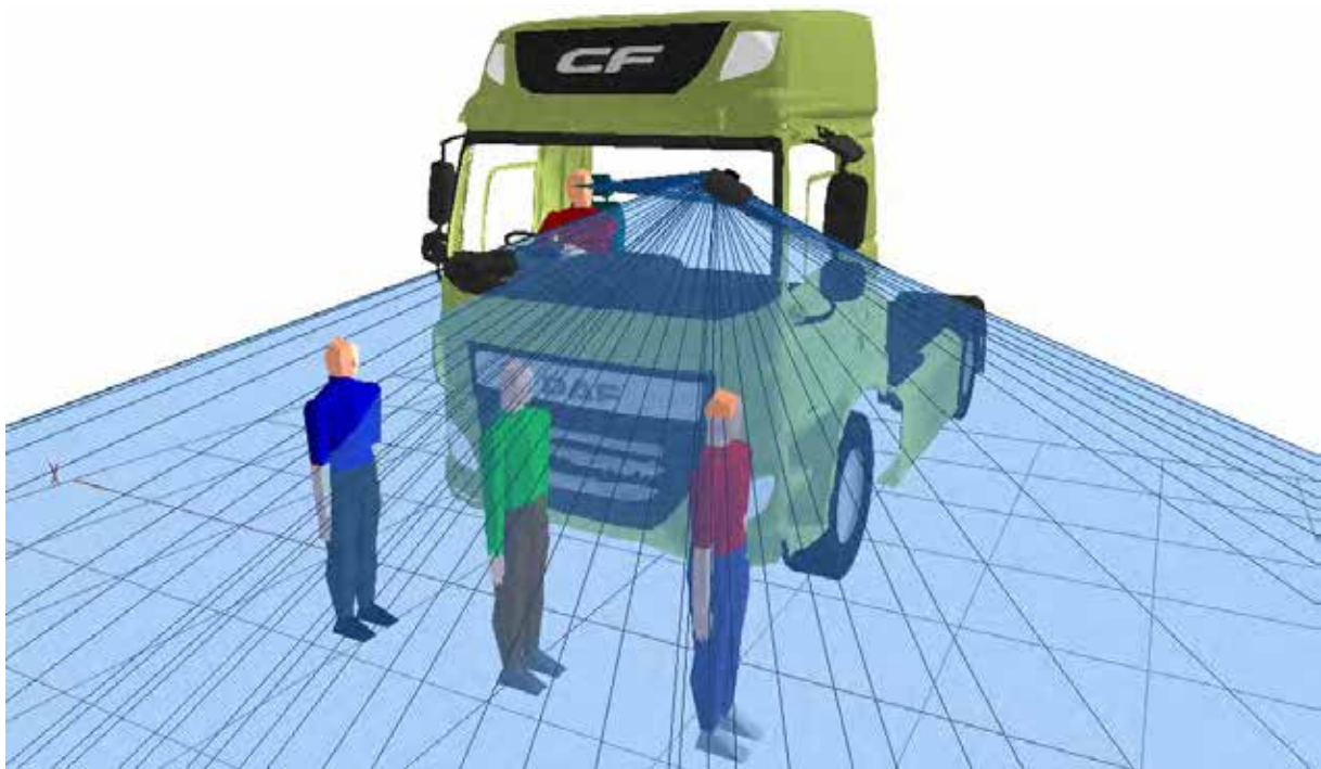
Figure 92. 3D view showing that all three pedestrians positioned to the front of the vehicle are visible in the projection of the Class VI mirror
