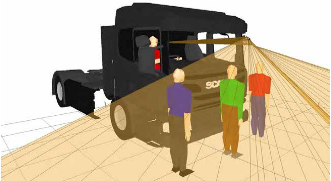
Figure 507. 3D view showing that all three pedestrians positioned to the front of the vehicle are visible in the projection of the Class VI mirror
