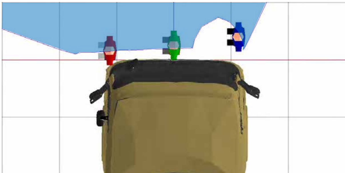
Figure 535. A plan view of the three human models that represent a pedestrian walking in front of a stationary vehicle and the projection of the windscreen at a height that equals the stature of a 50th%ile UK male pedestrian
