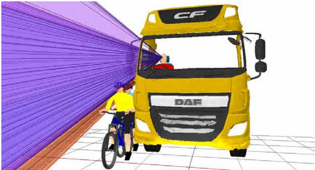
Figure 63. 3D view showing that both cyclists cannot be hidden from direct vision to the offside of the DAF CF N3
