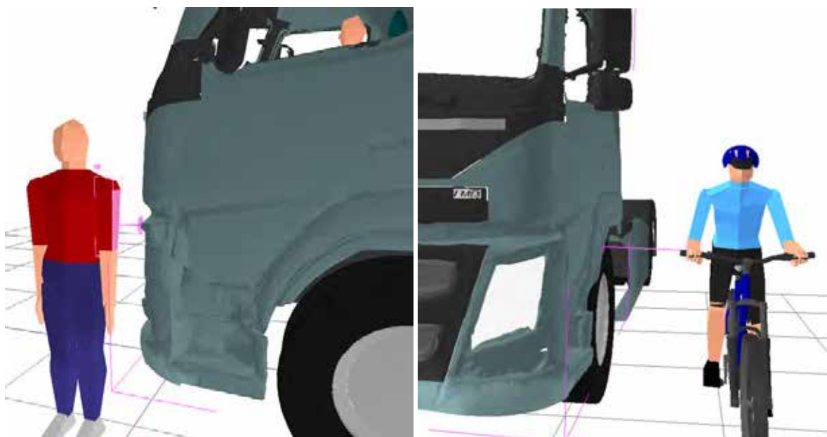
Figure 30. Measurement of shortest distance of a non-visible VRU to the test vehicle
