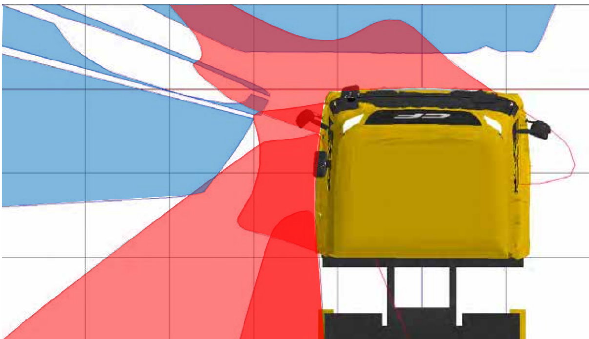
Figure 68. The areas of intersection of the projections of the driver’s field of view through windows and mirrors. The blue areas show the projection of the windscreen and the nearside windows, the red areas show the projection of the Class II, Class IV, Class V and Class VI mirrors, at a height above the ground that equals the height of a 50th%ile UK male cyclist
