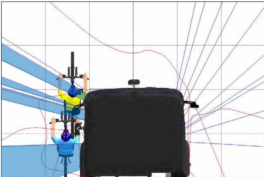
Figure 388. A plan view of the two human models that represent a cyclist moving up the inside of the vehicle and the projection of the windscreen and nearside windows at a height that equals the stature of a 50th%ile UK male cyclist
