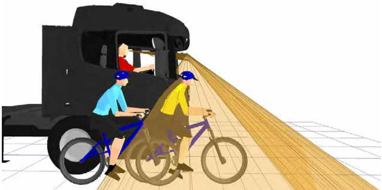
Figure 513. 3D view showing that the front (yellow) cyclist positioned to the offside of the vehicle is visible in the projection of the Class VI
