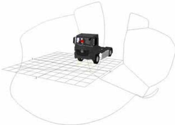
Figure 802. Combined indirect FOV area projection for the Mercedes Antos N3 / Arocs N3G / Actros N3
