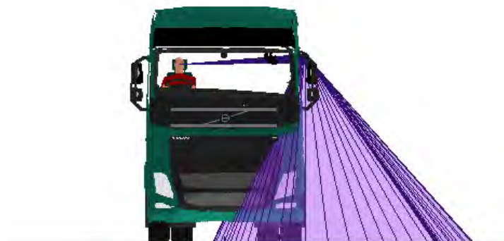
Figure 594. A front view of the Class V mirror projection for the Volvo FH N3
