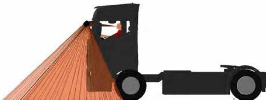
Figure 242. A side view of the Class VI mirror projection for the MAN TGX N3
