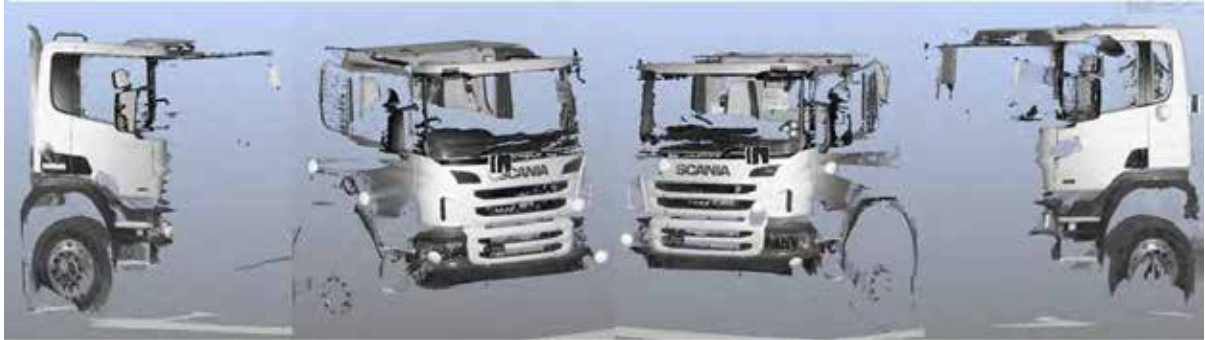
Figure 3. Example exterior scans showing the reference spheres which are used to combine four scan into one vehicle object
