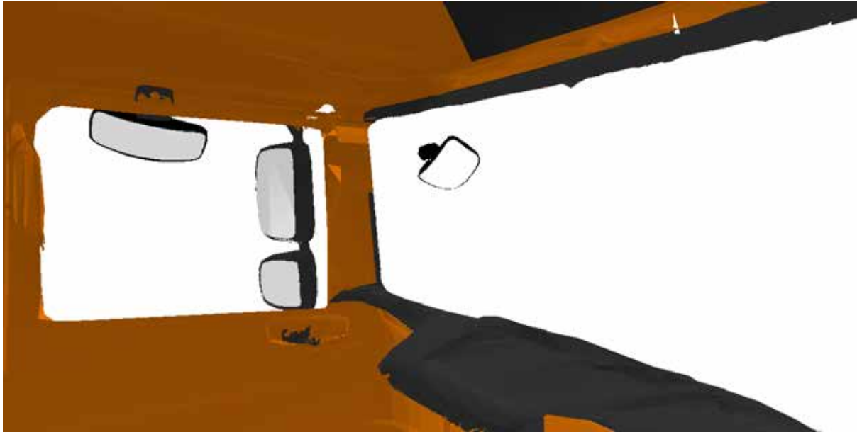
Figure 135. The view from the driver's eyes clearly shows the two cyclists are hidden from view.
