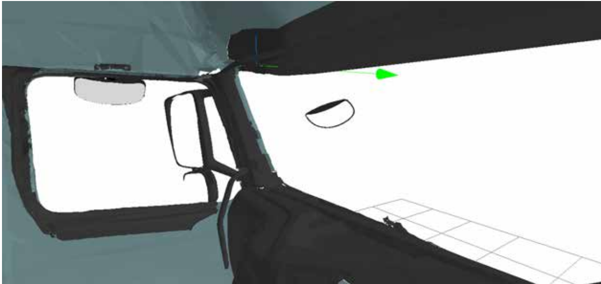
Figure 582. The view from the driver's eyes clearly shows the two cyclists are hidden from view.
