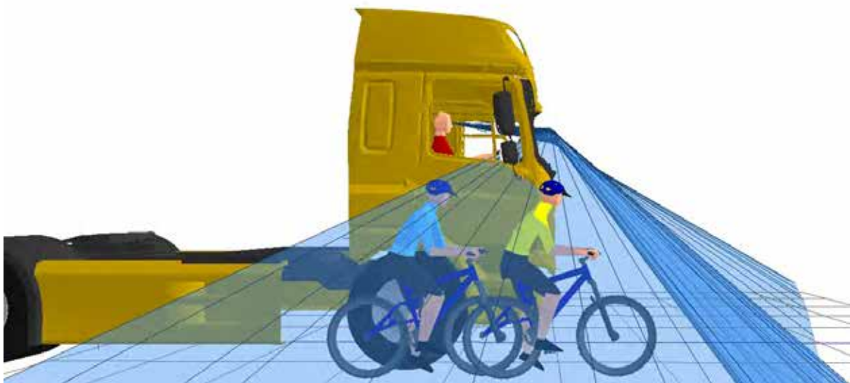
Figure 66. 3D view showing that the front (yellow) cyclist positioned to the offside of the vehicle is visible in the projection of the Class VI
