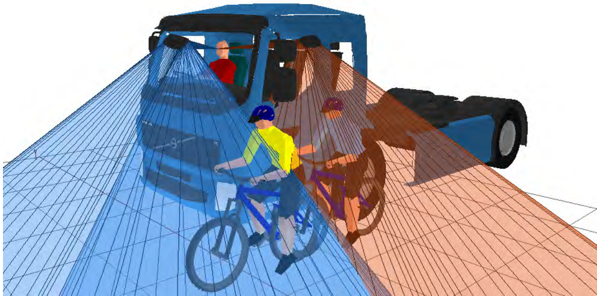
Figure 649. 3D view showing that both cyclists positioned to the nearside of the vehicle are visible in the projection of the Class V and / or Class VI mirrors
