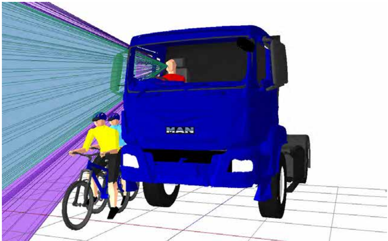
Figure 191. 3D view showing that both cyclists can be hidden from direct vision to the offside of the MAN TGS N3
