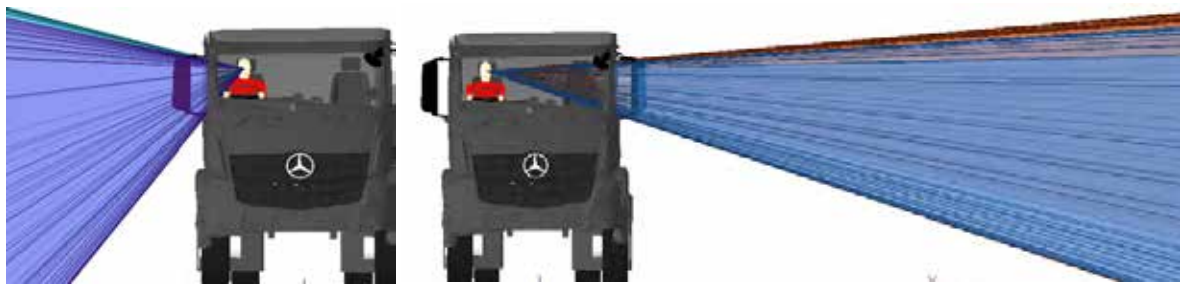
Figure 304. Frontal views of the off side and near side door window projections for the Mercedes Arocs N3G
