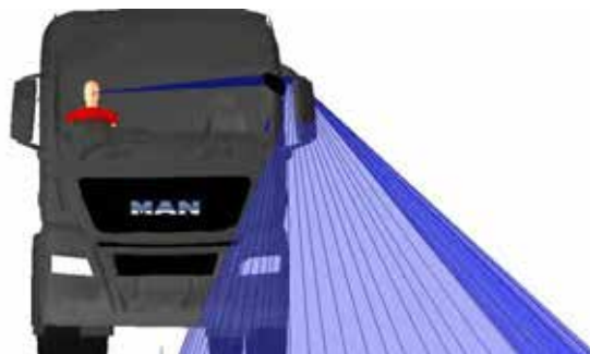
Figure 243. A front view of the Class V mirror projection for the MAN TGX N3
