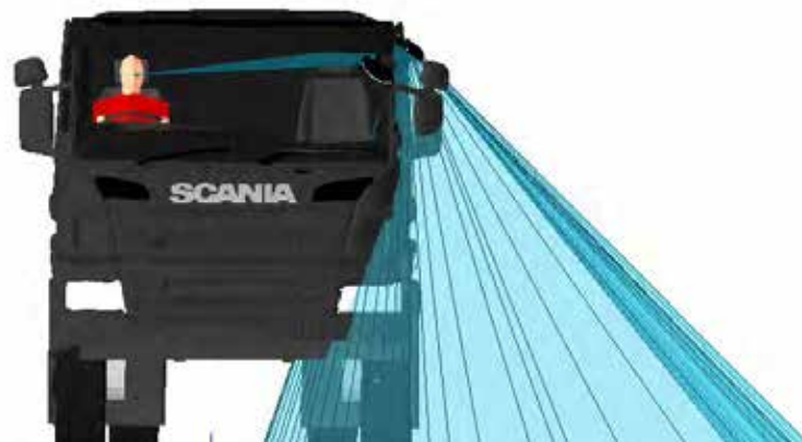
Figure 434. A front view of the Class V mirror projection for the Scania P N3G
