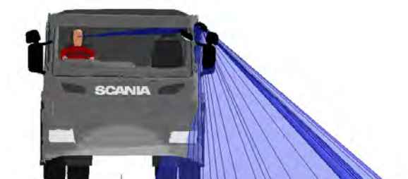
Figure 402. A front view of the Class V mirror projection for the Scania P N3
