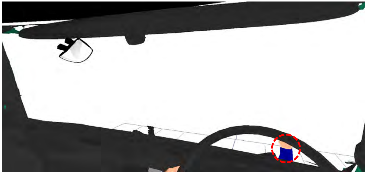
Figure 601. The view from the driver's eyes shows that all three pedestrians are hidden from view, though the right (blue) pedestrian may be visible through the centre of the steering wheel depending on its design.
