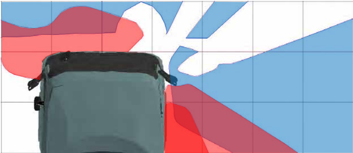
Figure 572. Image showing the areas of intersection of the projections of the driver's field of view through windows and mirrors. The blue areas show the projection of the windscreen and the offside windows, the red areas show the projection of the Class II, Class IV and Class VI mirrors, at a height above the ground that equals the height of a 50th%ile UK male cyclist
