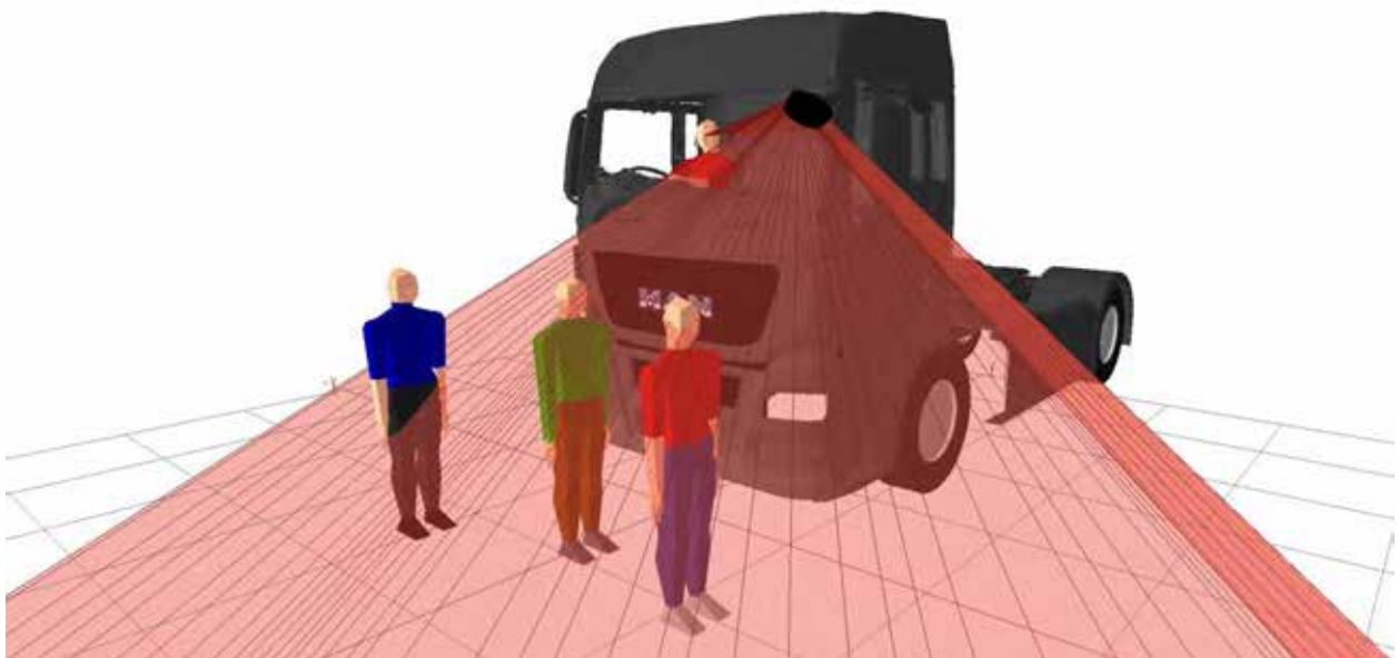
Figure 252. 3D view showing that all three pedestrians positioned to the front of the vehicle are visible in the projection of the Class VI mirror
