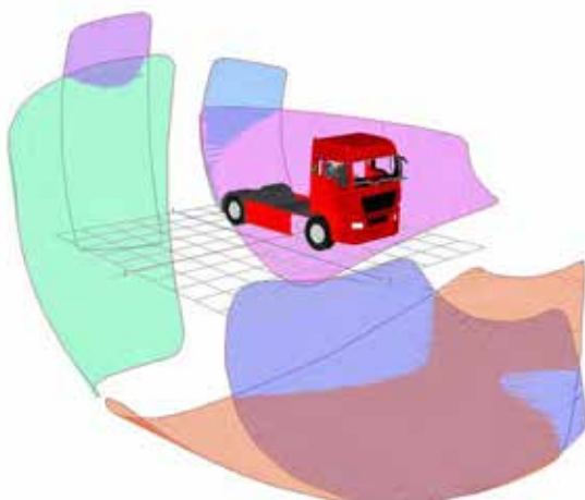
Figure 788. Indirect FOV area projection for the MAN TGX N3 / N3G
