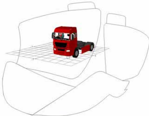
Figure 866. Combined indirect FOV area projection for the MAN TGX N3 / N3G
