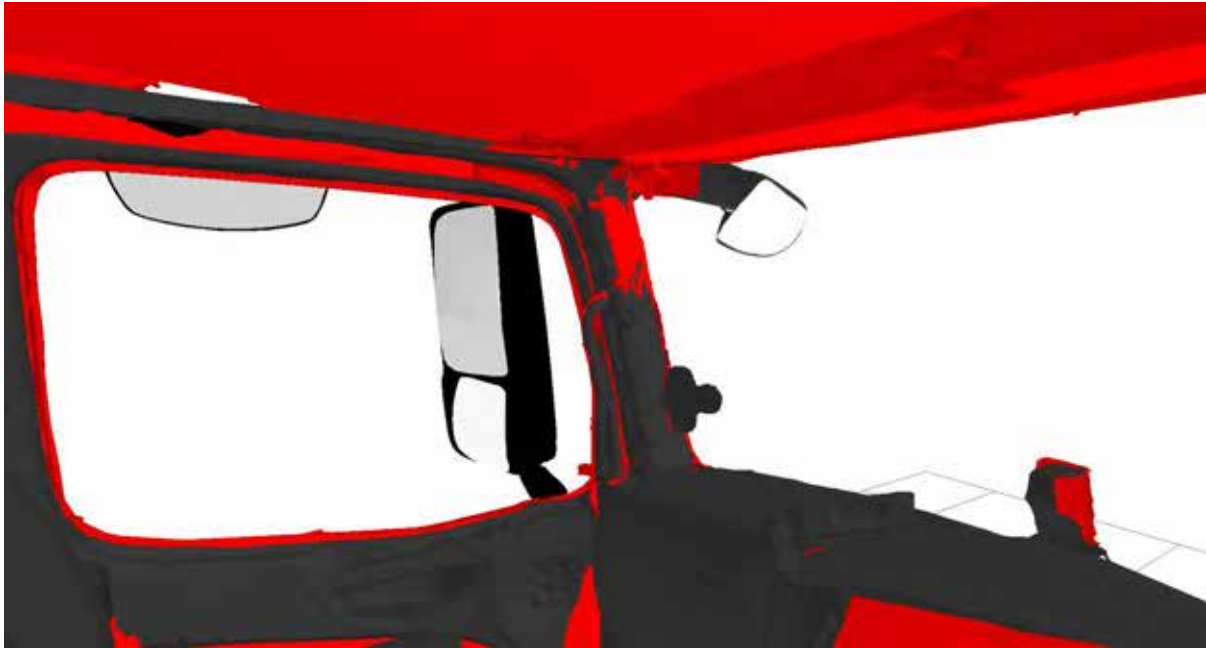
Figure 294. The view from the driver's eyes clearly shows the two cyclists are hidden from view.
