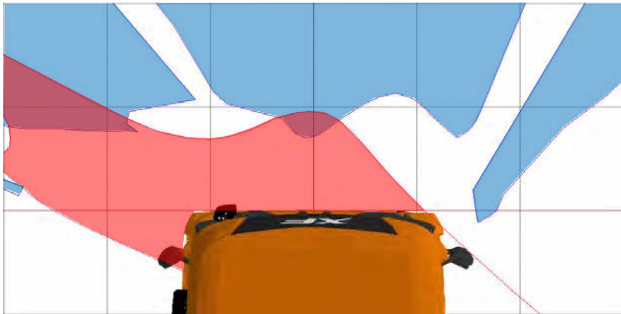
Figure 119. Image showing the areas of intersection of the projections of the driver’s field of view through windows and mirrors. The blue areas show the projection of the windscreen and part of the side windows, the red areas the projection of the Class VI mirror, at a height above the ground that equals the stature of a 50th%ile UK male pedestrian
