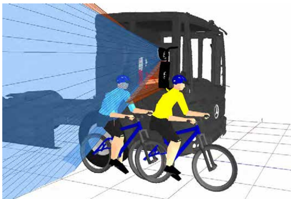
Figure 386. 3D view showing that the rear (blue) cyclist positioned to the offside of the vehicle is visible in the projection of the Class II mirror
