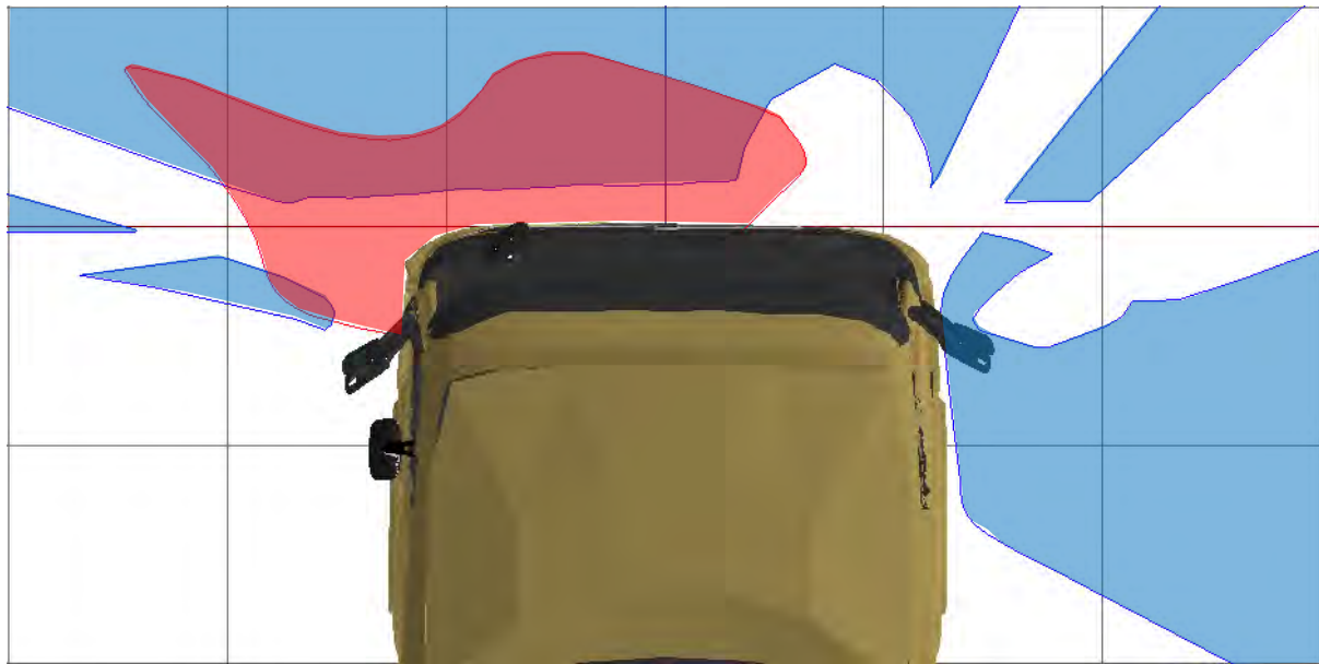
Figure 534. Image showing the areas of intersection of the projections of the driver’s field of view through windows and mirrors. The blue areas show the projection of the windscreen and part of the side windows, the red areas the projection of the Class VI mirror, at a height above the ground that equals the stature of a 50th%ile UK male pedestrian
