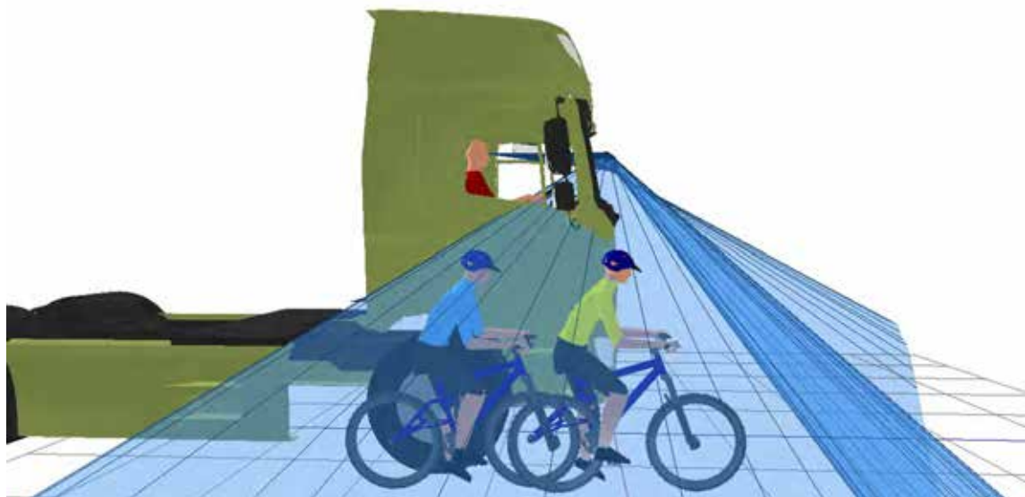
Figure 98. 3D view showing that the front (yellow) cyclist positioned to the offside of the vehicle is visible in the projection of the Class VI
