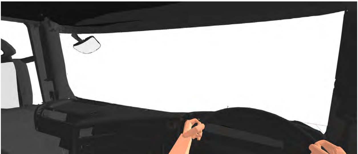
Figure 473. The view from the driver's eyes clearly shows the three pedestrians are hidden from view.
