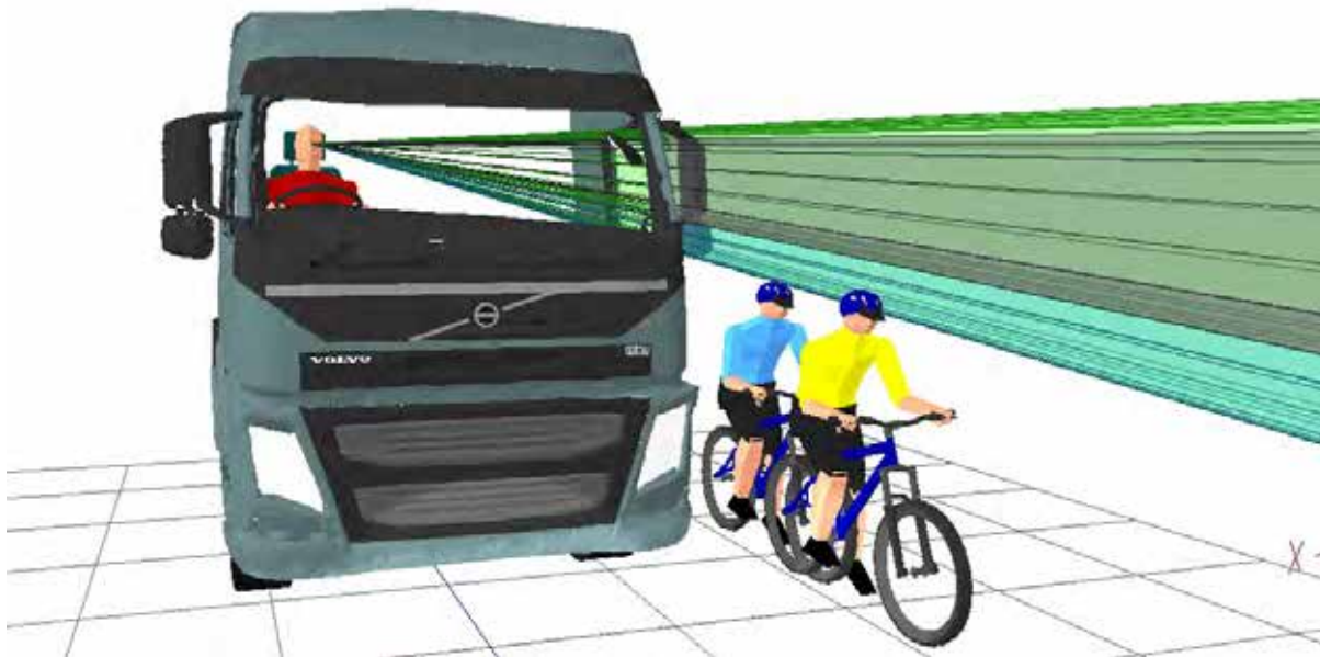
Figure 581. 3D view showing that the two human models can be positioned 462mm (yellow) and 526mm (blue) to the side of the vehicle without being seen through direct vision by the driver in the standardised driving posture
