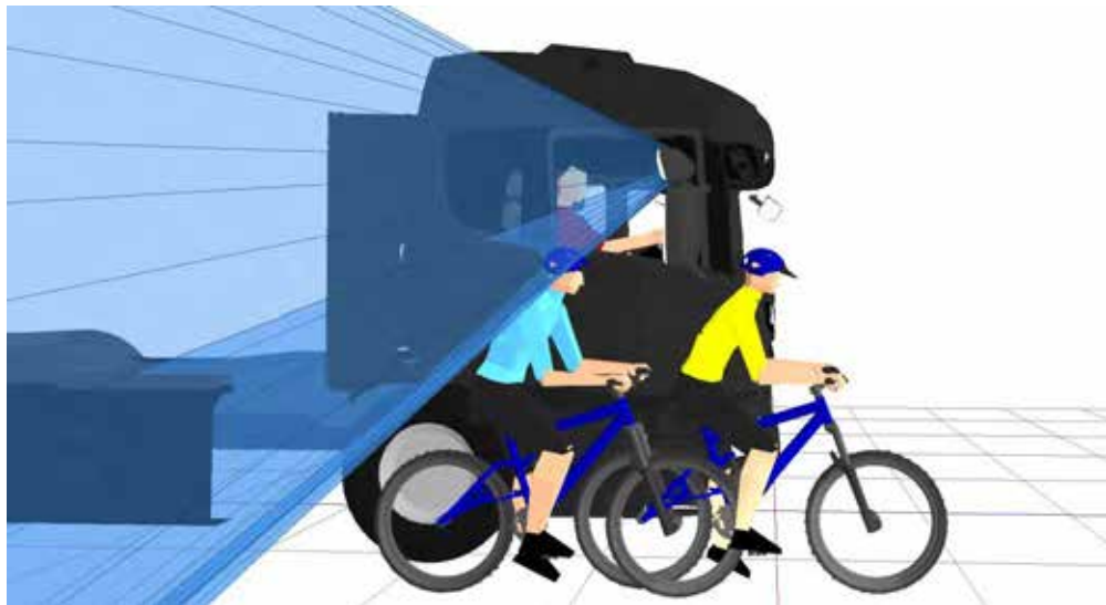
Figure 514. 3D view showing that the rear (blue) cyclist positioned to the offside of the vehicle is visible in the projection of the Class IV mirror
