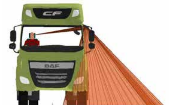
Figure 83. A front view of the Class V mirror projection for the DAF CF N3G
