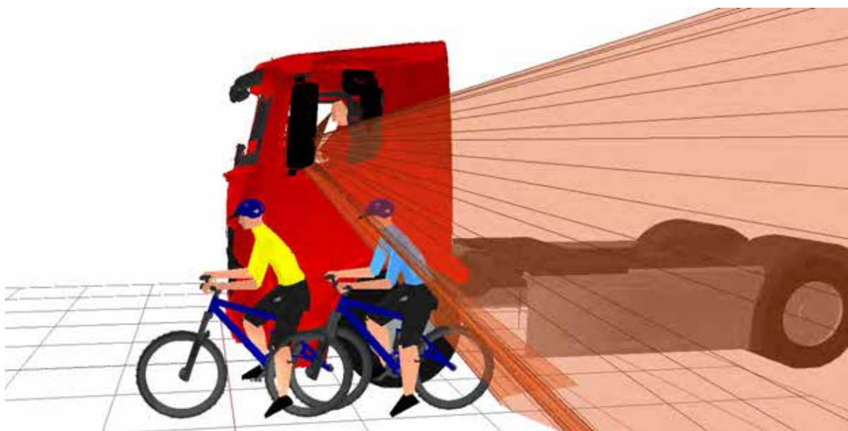
Figure 297. 3D view showing that the rear (blue) cyclist positioned to the nearside of the vehicle is visible in the projection of the Class IV mirror
