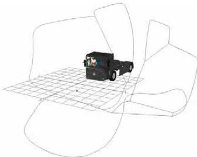
Figure 697. Combined indirect FOV area projection for the Mercedes Econic N3 LEC
