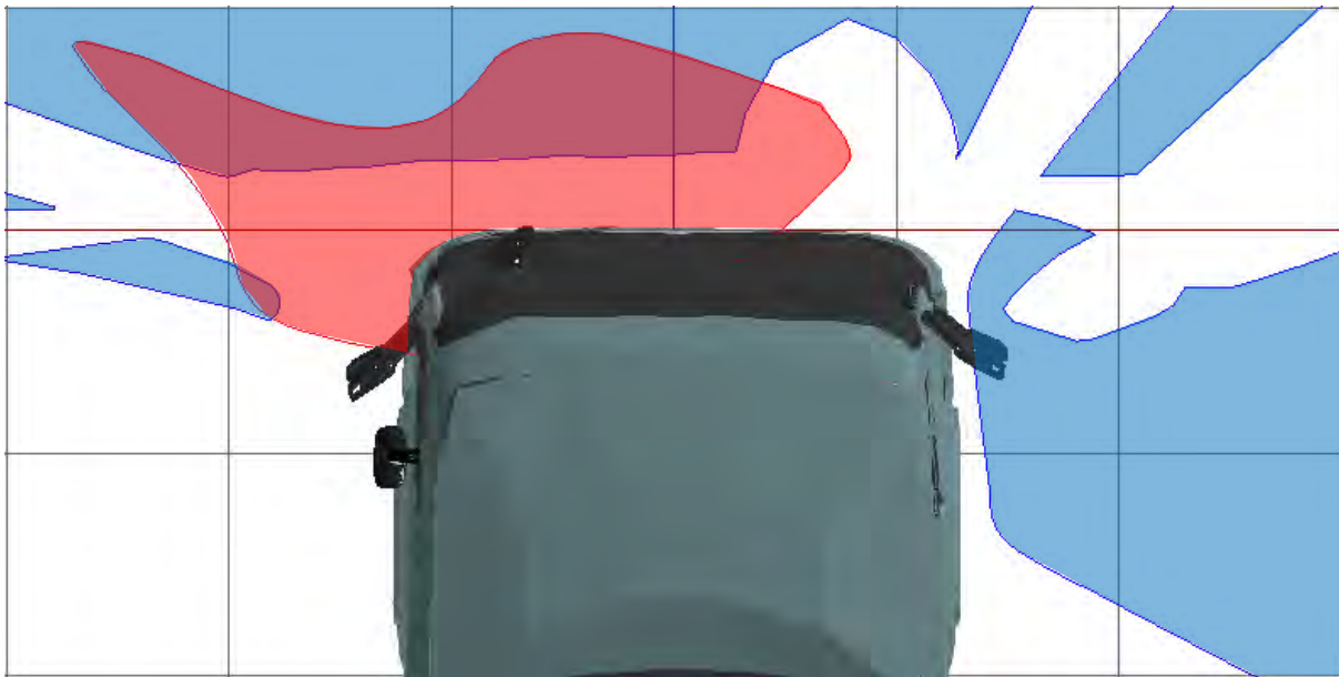
Figure 566. Image showing the areas of intersection of the projections of the driver’s field of view through windows and mirrors. The blue areas show the projection of the windscreen and part of the side windows, the red areas the projection of the Class VI mirror, at a height above the ground that equals the stature of a 50th%ile UK male pedestrian
