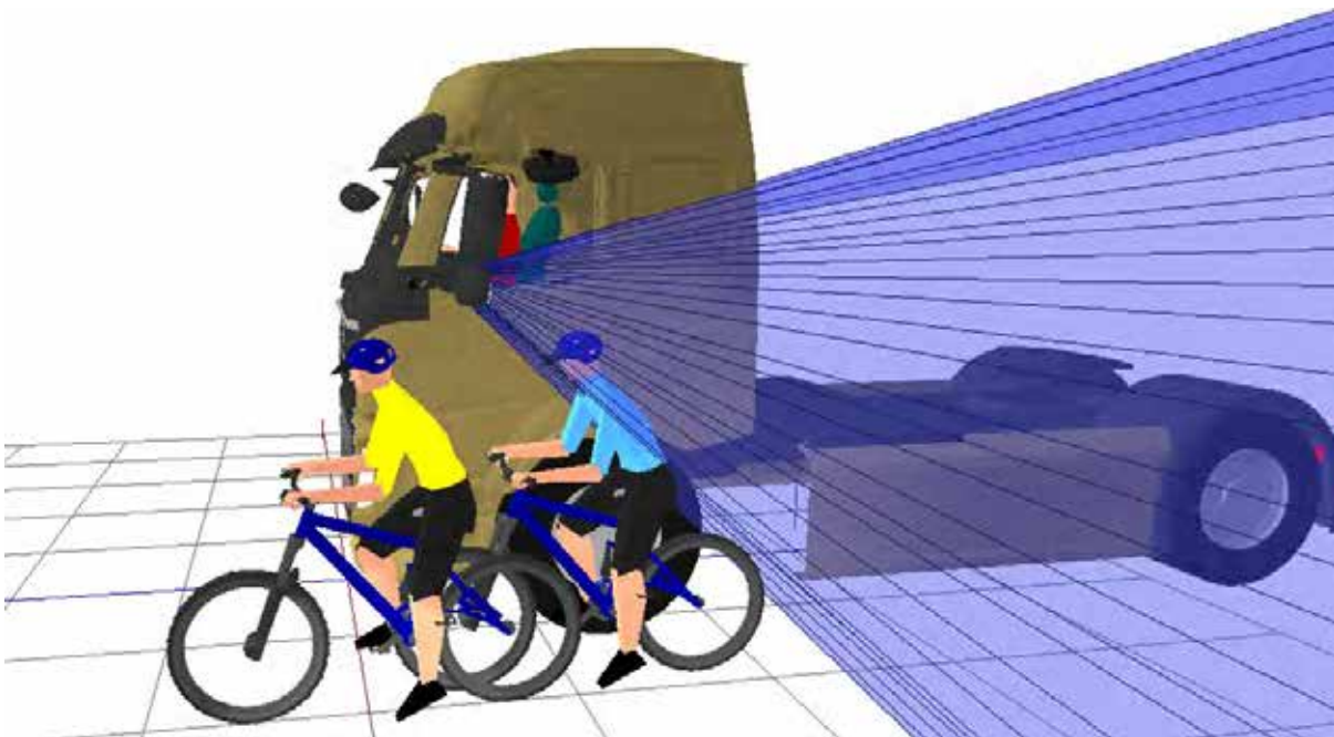
Figure 553. 3D view showing that the rear (blue) cyclist positioned to the nearside of the vehicle is visible in the projection of the Class IV mirror
