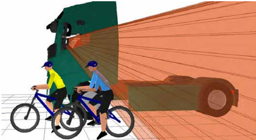
Figure 618. 3D view showing that the rear (blue) cyclist positioned to the nearside of the vehicle is barely visible in the projection of the Class IV mirror
