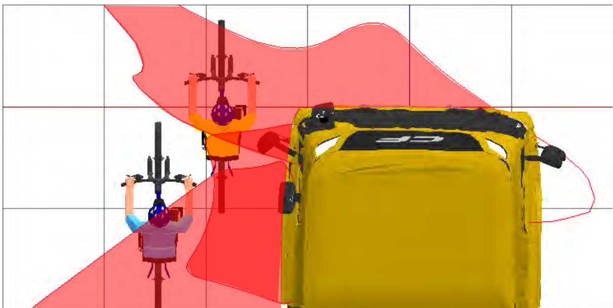
Figure 72. A plan view of the two human models that represent a cyclist moving up the inside of the vehicle and the projection of the Class IV, Class V and Class VI mirrors at a height that equals the stature of a 50th%ile UK male cyclist
