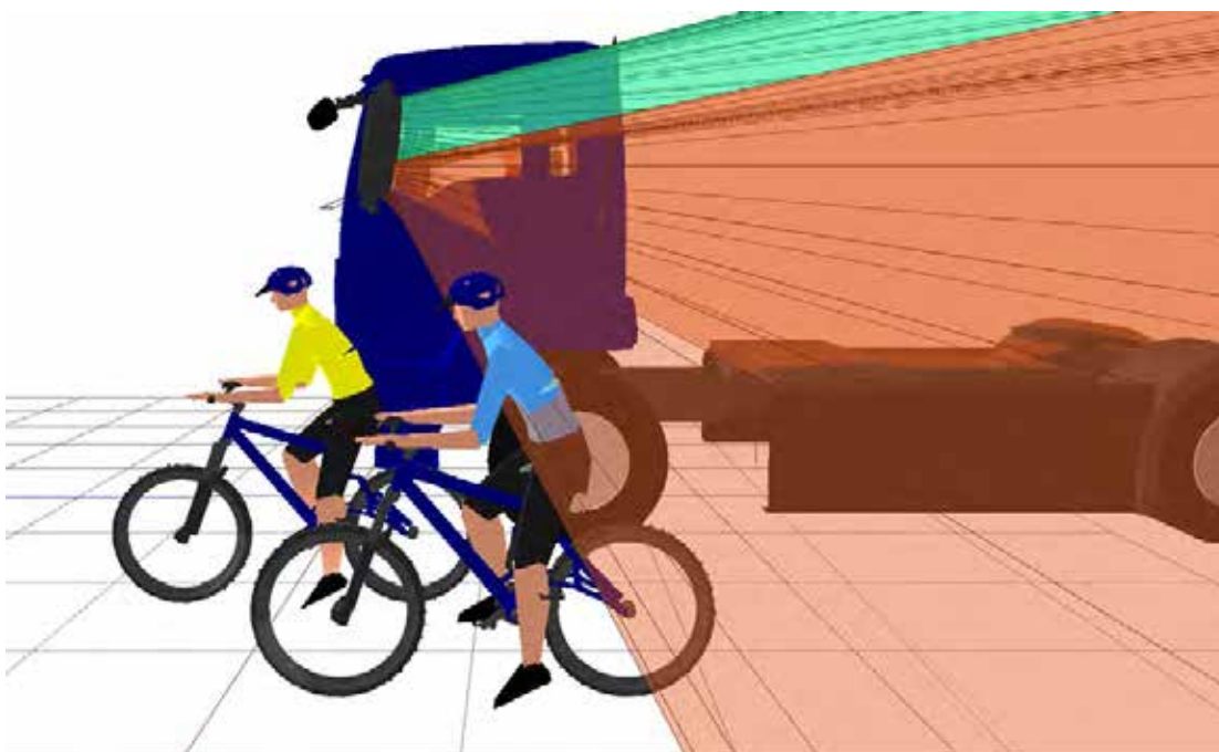
Figure 202. 3D view showing that the rear (blue) cyclist positioned to the nearside of the vehicle is visible in the projection of the Class IV mirror
