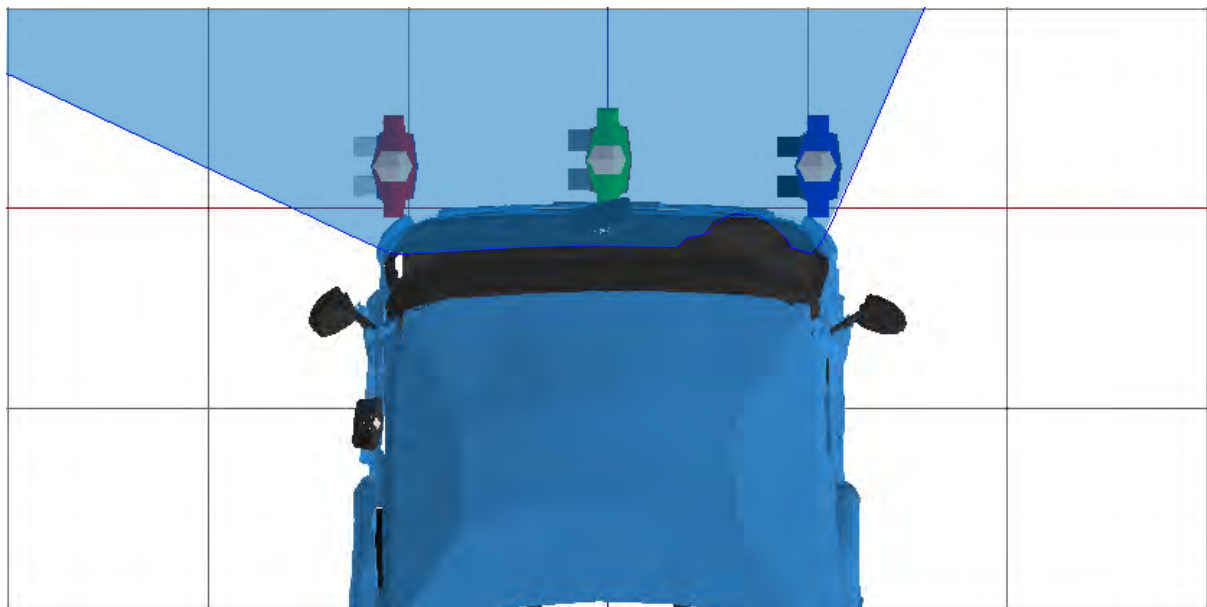
Figure 632. A plan view of the three human models that represent a pedestrian walking in front of a stationary vehicle and the projection of the windscreen at a height that equals the stature of a 50th%ile UK male pedestrian
