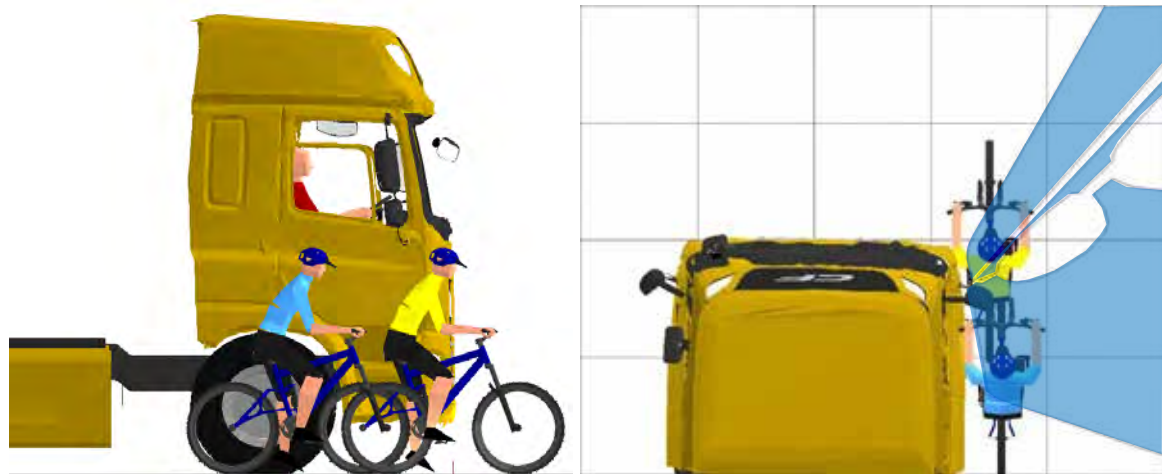
Figure 25. The configuration of the cyclist models positioned to the offside of the vehicle. The image to the left shows a view to the offside of the vehicle. The image to the right shows a plan (top-down) view.
