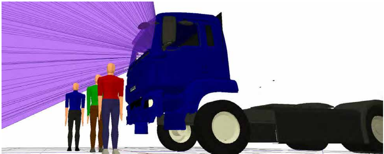
Figure 185. 3D view showing that the three human models can stand 1122mm (blue), 613mm (green) and 546mm (red) in front of the vehicle without being seen through direct vision by the driver in the standardised driving posture
