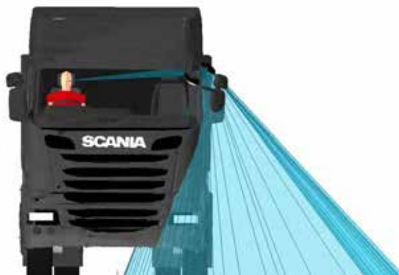
Figure 466. A front view of the Class V mirror projection for the Scania R N3
