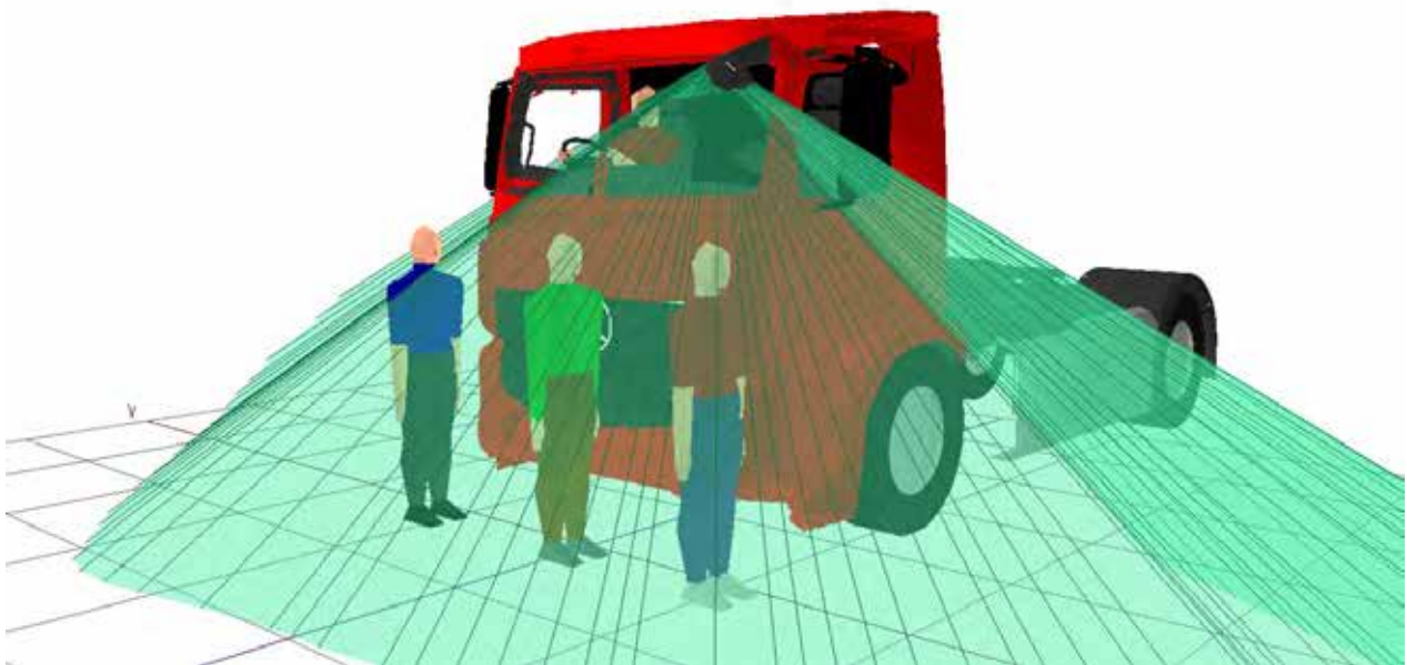
Figure 283. 3D view showing that all three pedestrians positioned to the front of the vehicle are visible in the projection of the Class VI mirror
