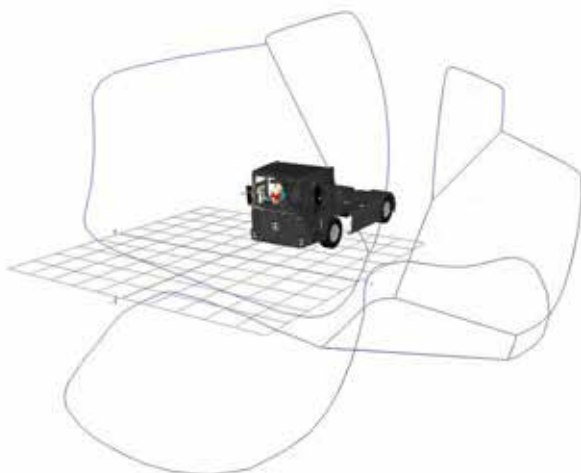
Figure 803. Combined indirect FOV area projection for the Mercedes Econic N3 LEC
