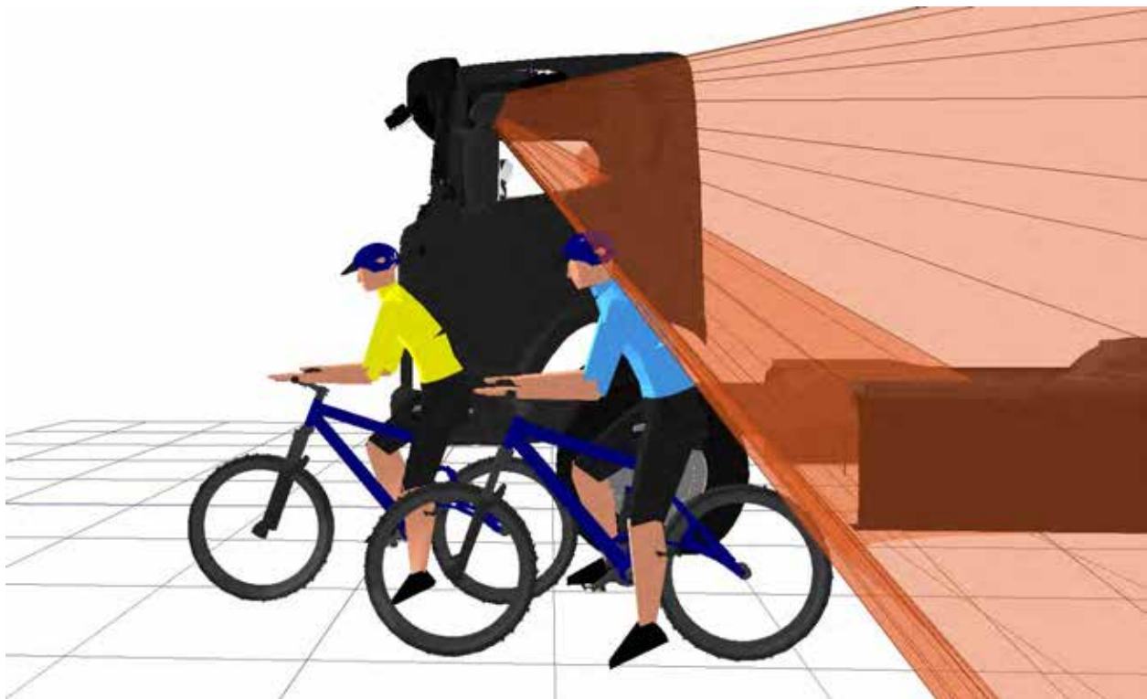
Figure 457. 3D view showing that the rear (blue) cyclist positioned to the nearside of the vehicle is not visible in the projection of the Class IV or Class II mirror
