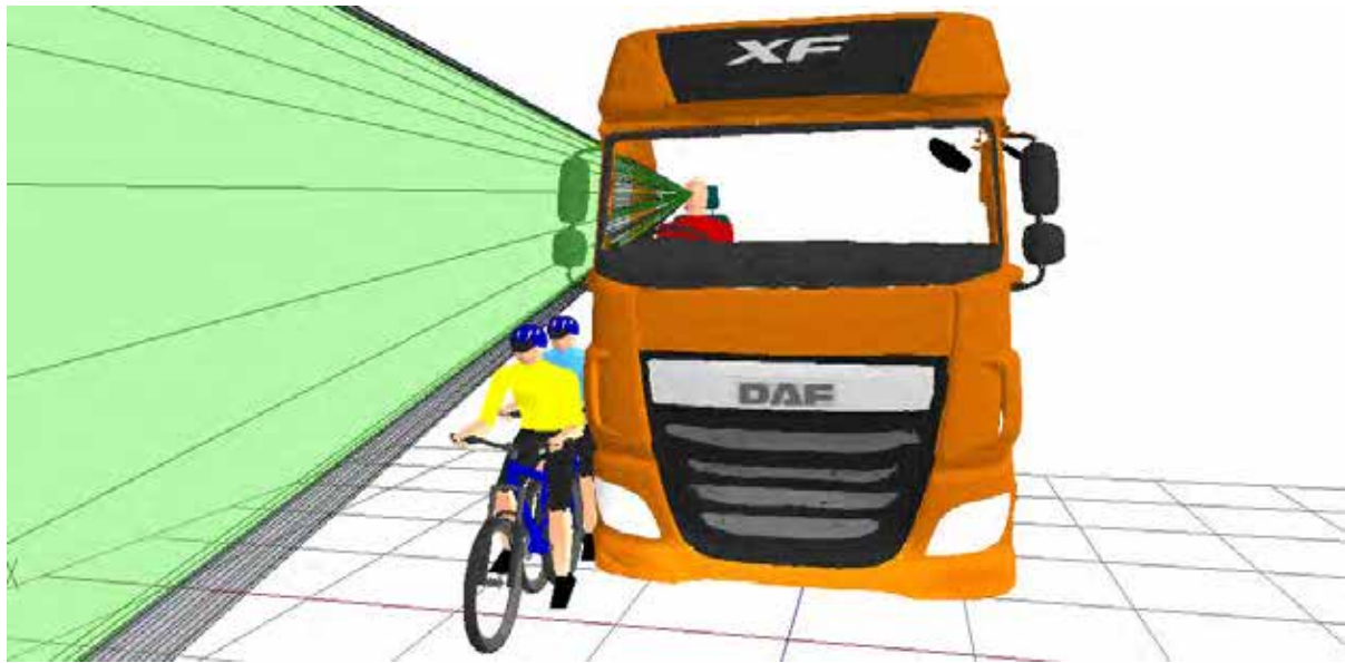
Figure 127. 3D view showing that the two human models can be positioned 0mm (yellow) and 53mm (blue) to the side of the vehicle without being seen through direct vision by the driver in the standardised driving posture
