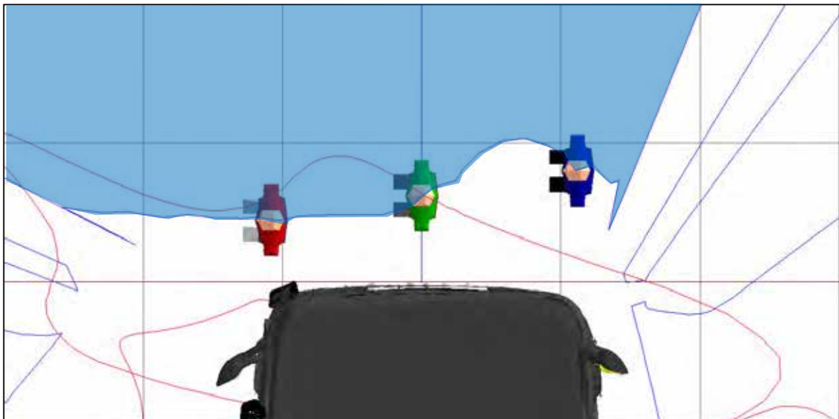
Figure 471. A plan view of the three human models that represent a pedestrian walking in front of a stationary vehicle and the projection of the windscreen at a height that equals the stature of a 50th%ile UK male pedestrian
