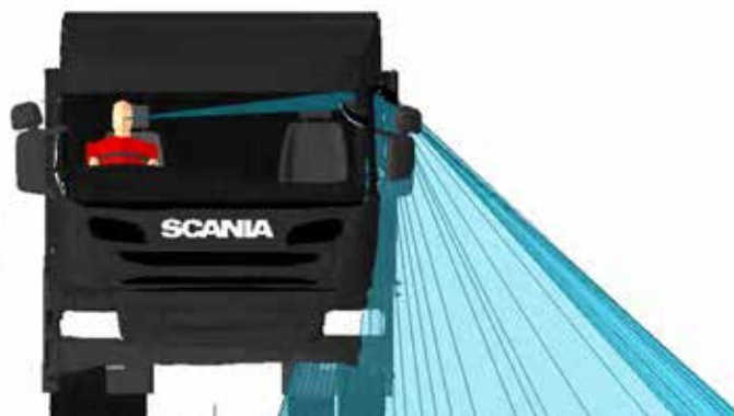
Figure 498. A front view of the Class V mirror projection for the Scania N3 LEC
