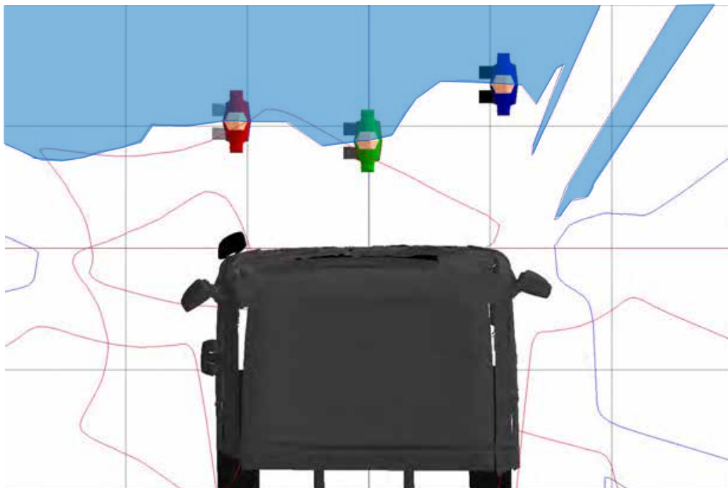
Figure 248. A plan view of the three human models that represent a pedestrian walking in front of a stationary vehicle and the projection of the windscreen at a height that equals the stature of a 50th%ile UK male pedestrian
