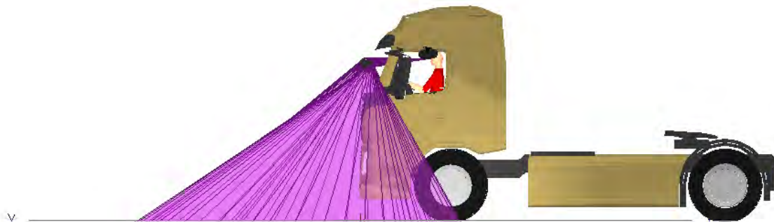
Figure 529. A side view of the Class VI mirror projection for the Volvo FM N3
