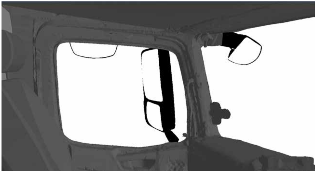
Figure 358. The view from the driver's eyes clearly shows the two cyclists are hidden from view.
