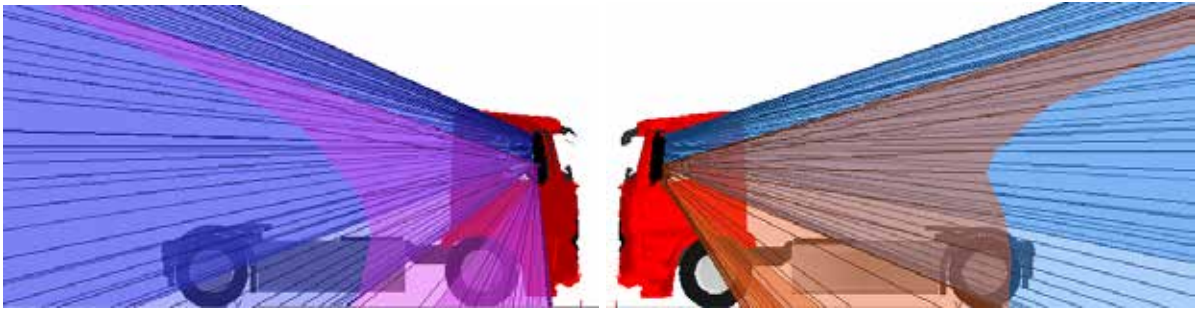
Figure 275. Side views of the combined Class II and Class IV mirror projections for the Mercedes Antos N3
