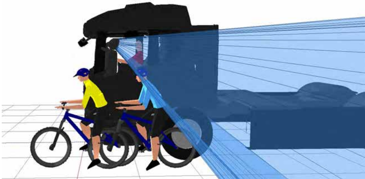
Figure 521. 3D view showing that the rear (blue) cyclist positioned to the nearside of the vehicle is visible in the projection of the Class IV mirror
