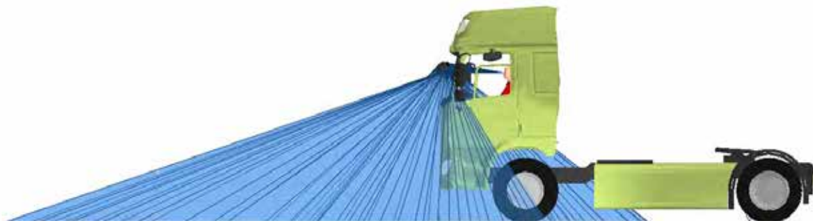
Figure 82. A side view of the Class VI mirror projection for the DAF CF N3G
