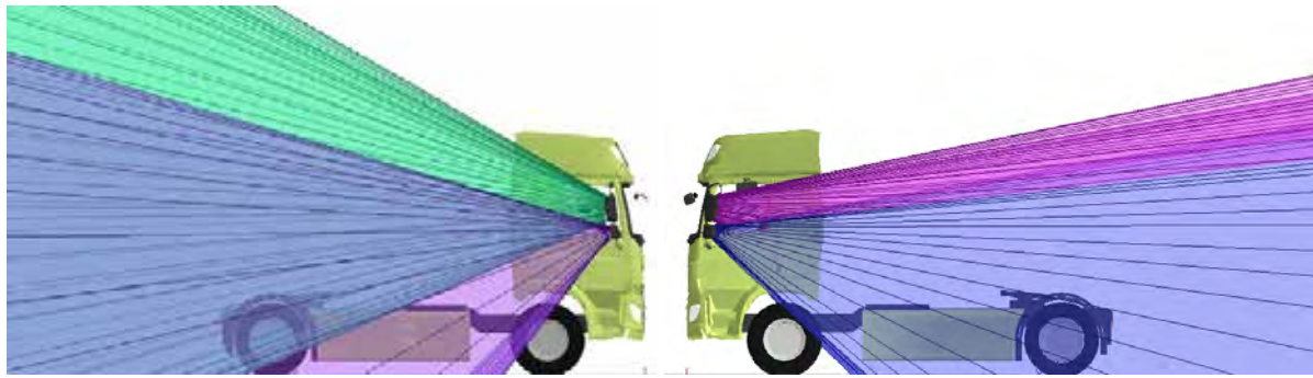
Figure 84. Side views of the combined Class II and Class IV mirror projections for the DAF CF N3G
