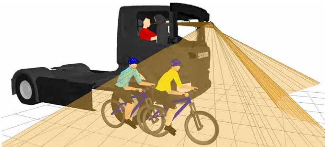
Figure 449. 3D view showing that the front (yellow) cyclist positioned to the offside of the vehicle is visible in the projection of the Class VI
