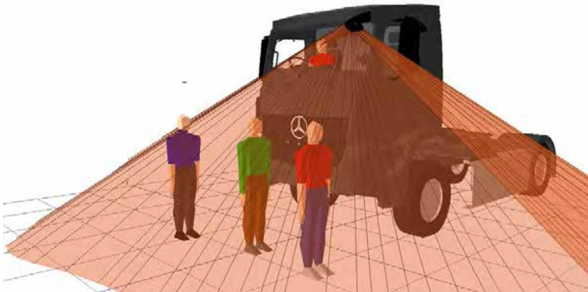
Figure 315. 3D view showing that all three pedestrians positioned to the front of the vehicle are visible in the projection of the Class VI mirror
