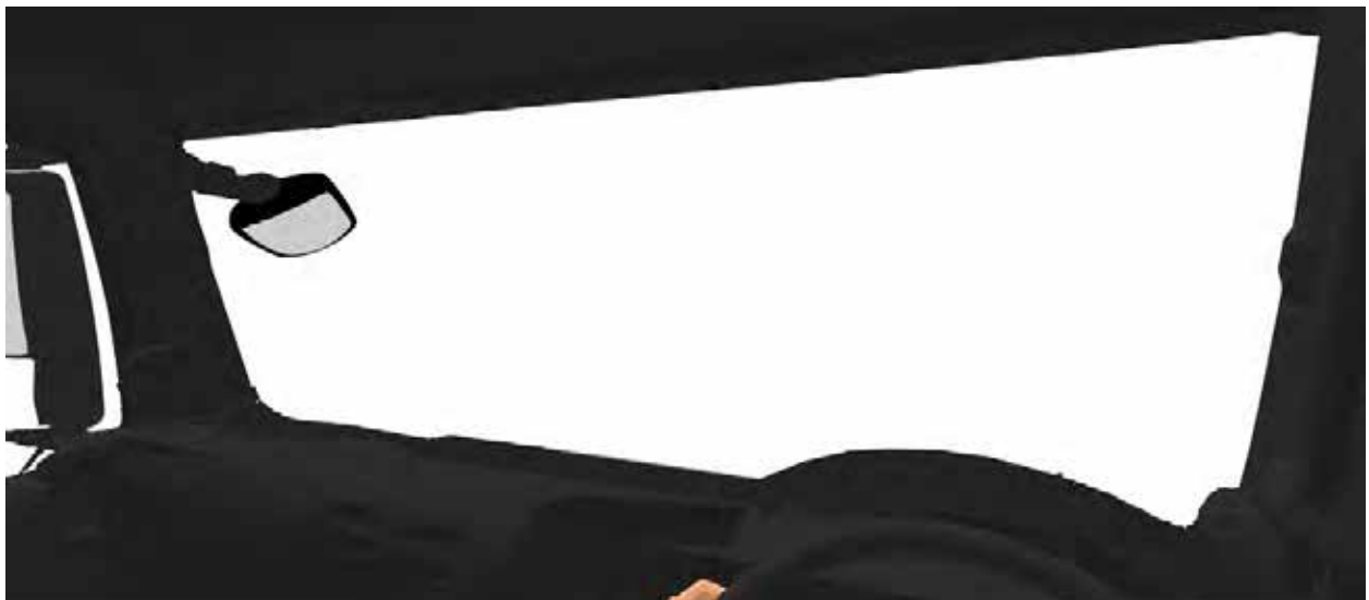
Figure 218. The view from the driver's eyes clearly shows the three pedestrians are hidden from view.
