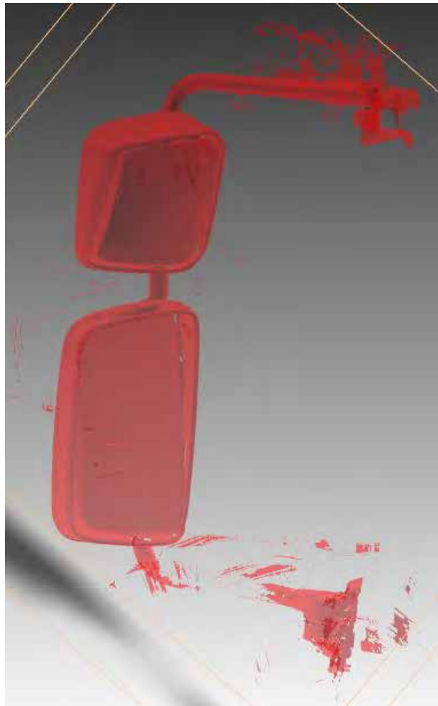
Figure 5. An example of the data that was captured from a mirror arm holding the Class II and Class IV mirrors, using a ZCORP Hand laser scanner
