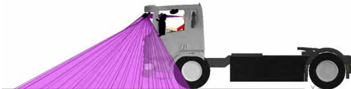
Figure 401. A side view of the Class VI mirror projection for the Scania P N3
