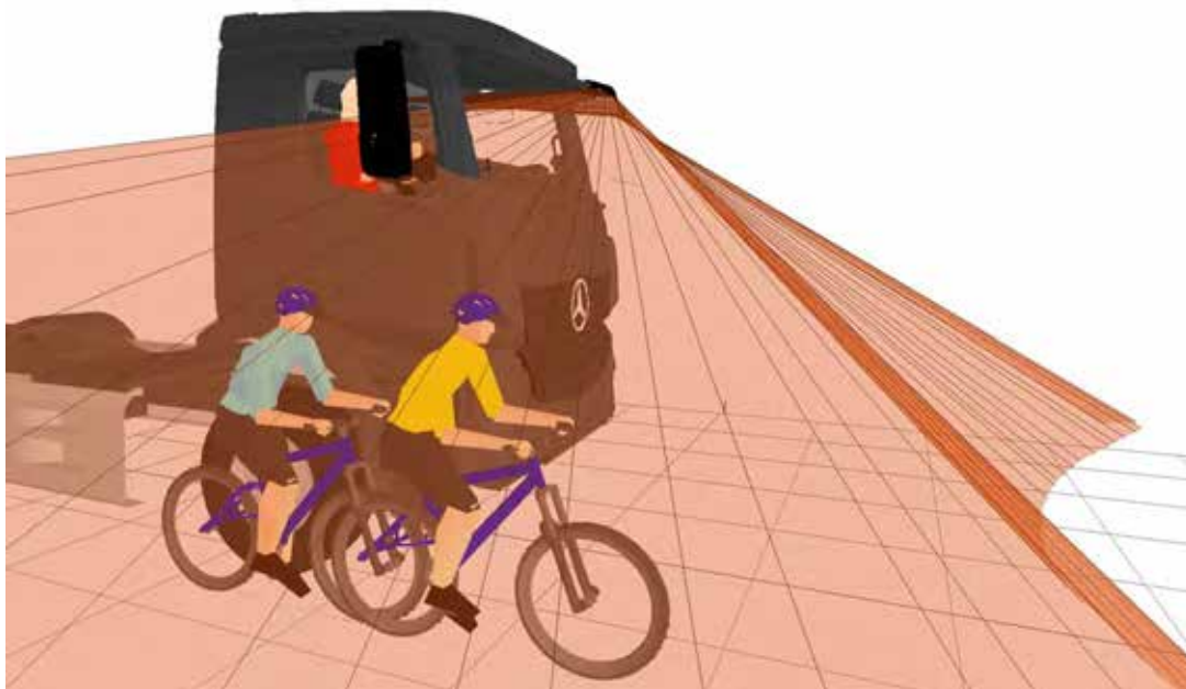
Figure 321. 3D view showing that the front (yellow) cyclist positioned to the offside of the vehicle is visible in the projection of the Class VI
