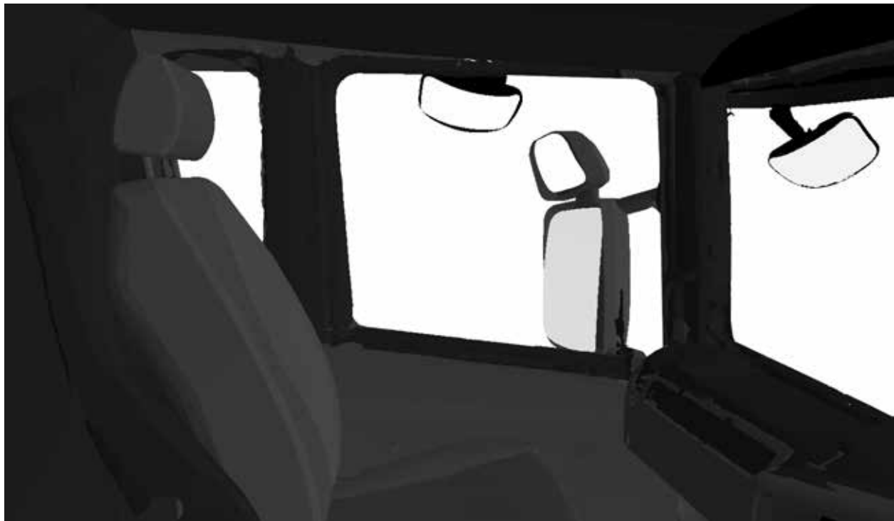
Figure 454. The view from the driver's eyes clearly shows the two cyclists are hidden from view.
