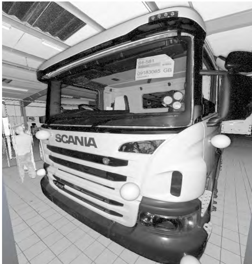
Figure 7. The scan of the taped windscreen to allow the visible area of the glass to capture and digitised
