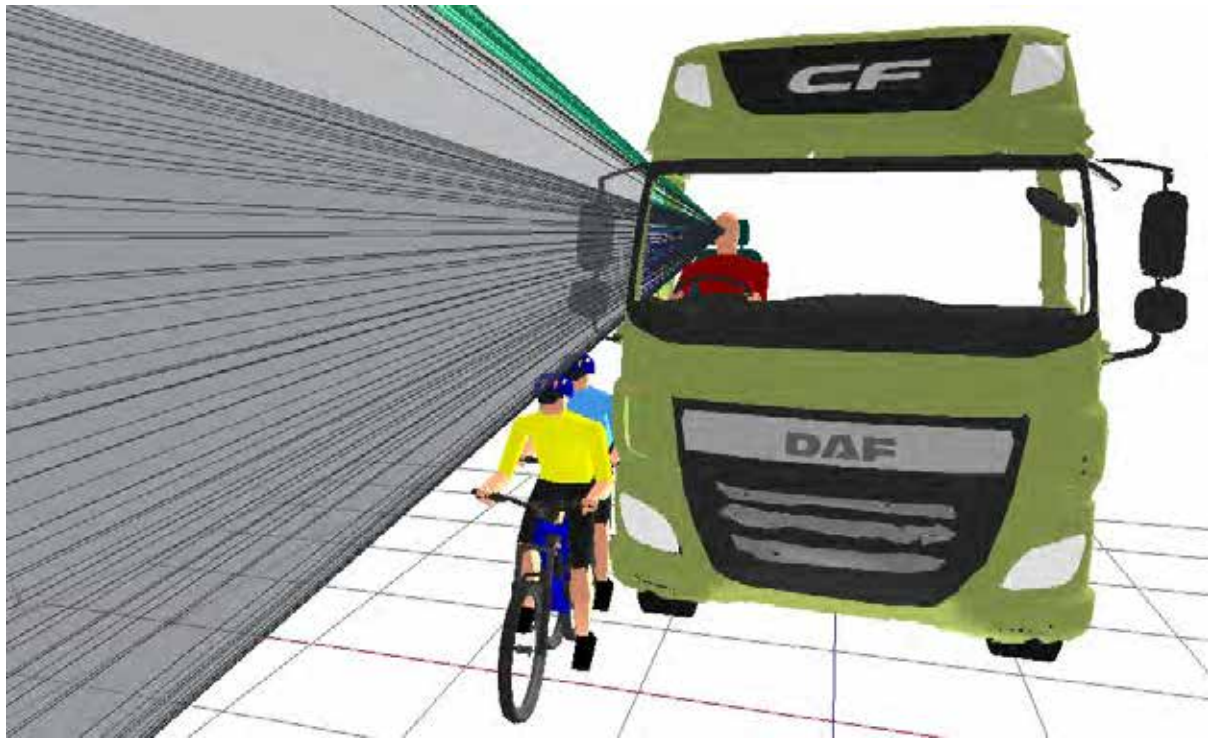
Figure 95. 3D view showing that both cyclists cannot be hidden from direct vision to the offside of the DAF CF N3
