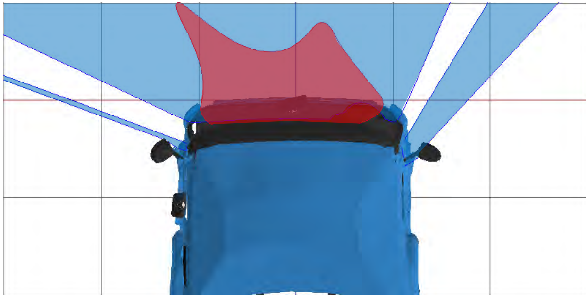
Figure 631. Image showing the areas of intersection of the projections of the driver’s field of view through windows and mirrors. The blue areas show the projection of the windscreen and part of the side windows, the red areas the projection of the Class VI mirror, at a height above the ground that equals the stature of a 50th%ile UK male pedestrian
