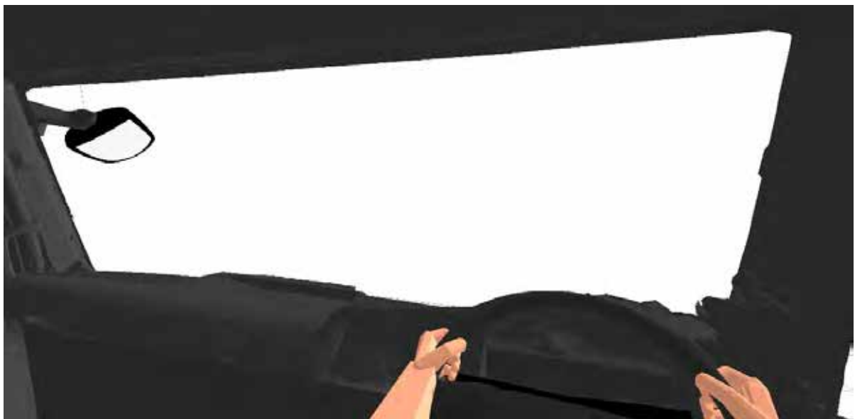
Figure 250. The view from the driver's eyes clearly shows the three pedestrians are hidden from view.
