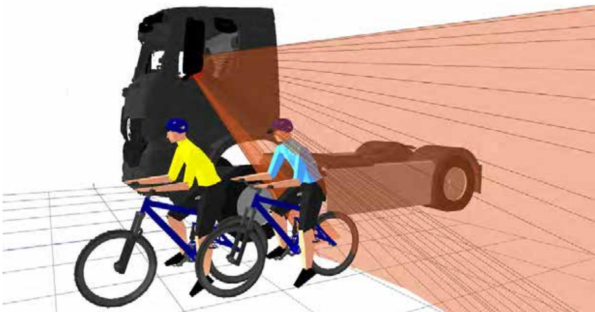
Figure 329. 3D view showing that the rear (blue) cyclist positioned to the nearside of the vehicle is partially visible in the Class IV mirror
