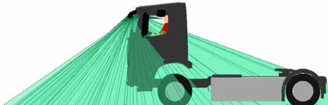
Figure 305. A side view of the Class VI mirror projection for the Mercedes Arocs N3G
