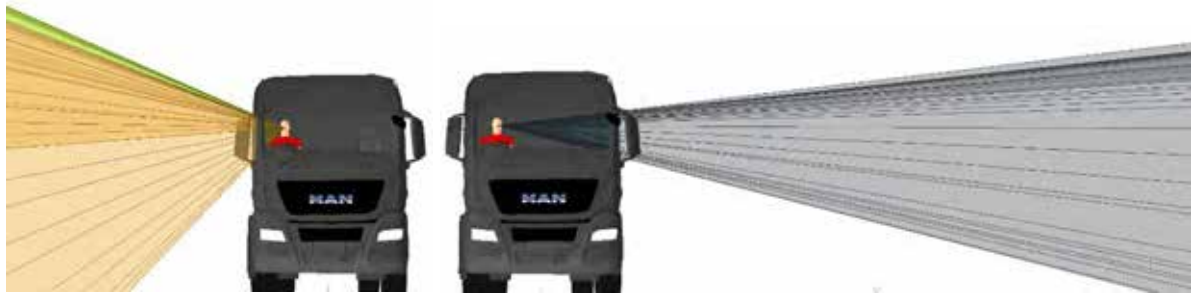
Figure 241. Frontal views of the off side and near side door window projections for the MAN TGX N3
