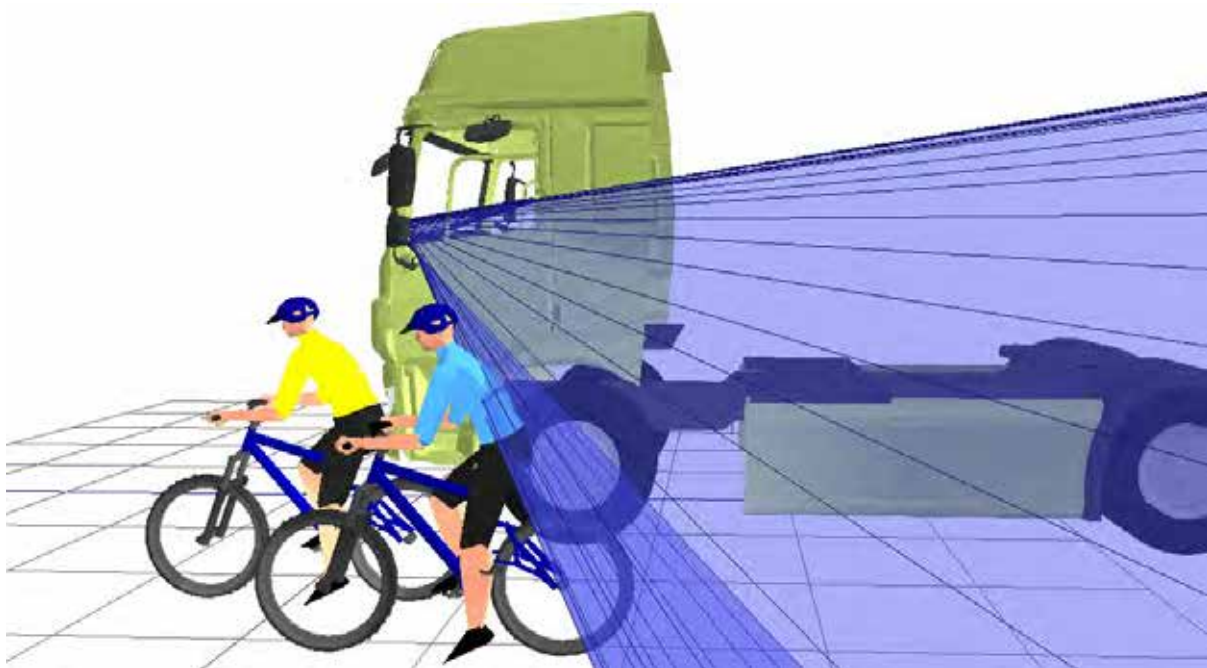
Figure 106. 3D view showing that the rear (blue) cyclist positioned to the nearside of the vehicle is barely visible in the projection of the Class IV mirror
