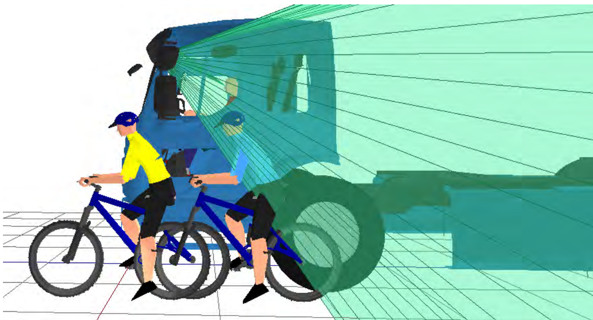
Figure 650. 3D view showing that the rear (blue) cyclist positioned to the nearside of the vehicle is visible in the projection of the Class IV mirror
