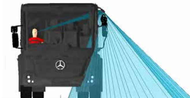
Figure 370. A front view of the Class V mirror projection for the Mercedes Econic LEC
