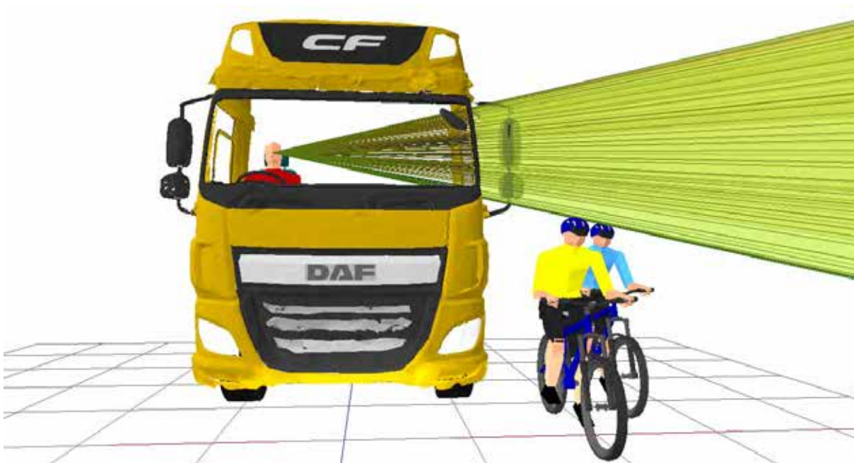
Figure 70. 3D view showing that the two human models can be positioned 230mm (yellow) and 848mm (blue) to the side of the vehicle without being seen through direct vision by the driver in the standardised driving posture
