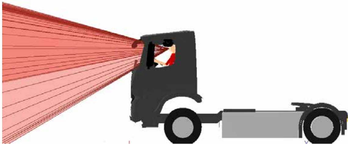
Figure 303. A side view of the windscreen aperture projection for the Mercedes Arocs N3G
