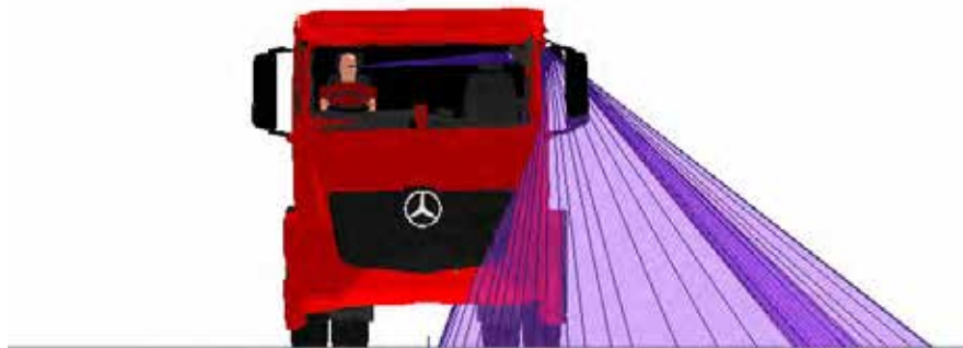
Figure 274. A front view of the Class V mirror projection for the Mercedes Antos N3
