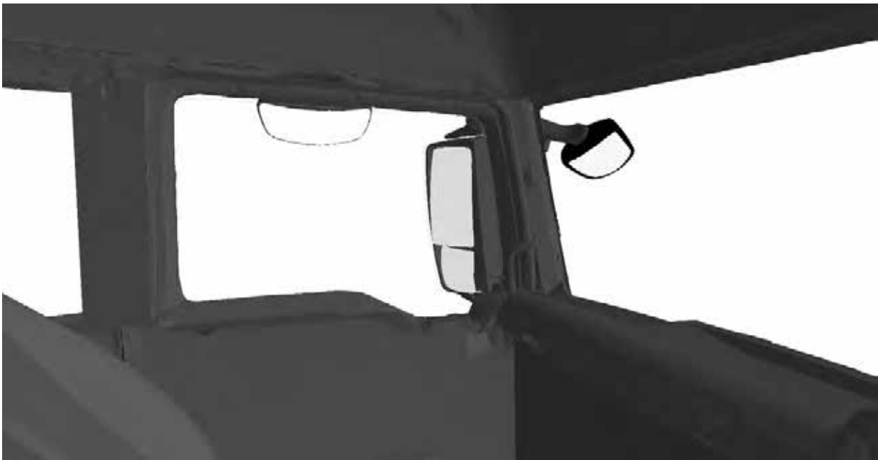
Figure 262. The view from the driver's eyes clearly shows the two cyclists are hidden from view.
