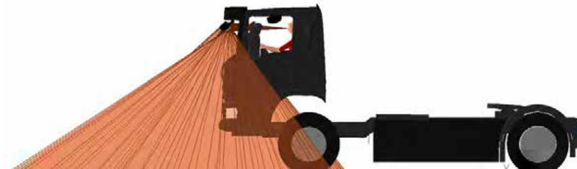
Figure 433. A side view of the Class VI mirror projection for the Scania P N3G
