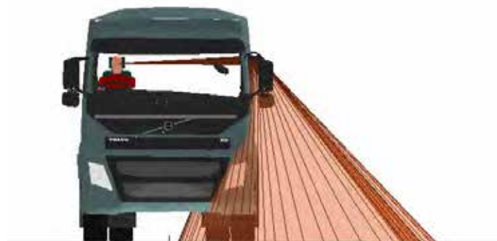
Figure 562. A front view of the Class V mirror projection for the Volvo FMX N3G
