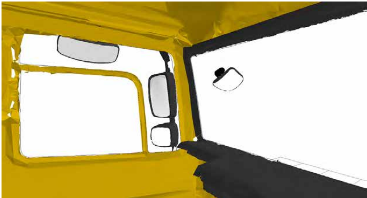
Figure 71. The view from the driver's eyes clearly shows the two cyclists are hidden from view.
