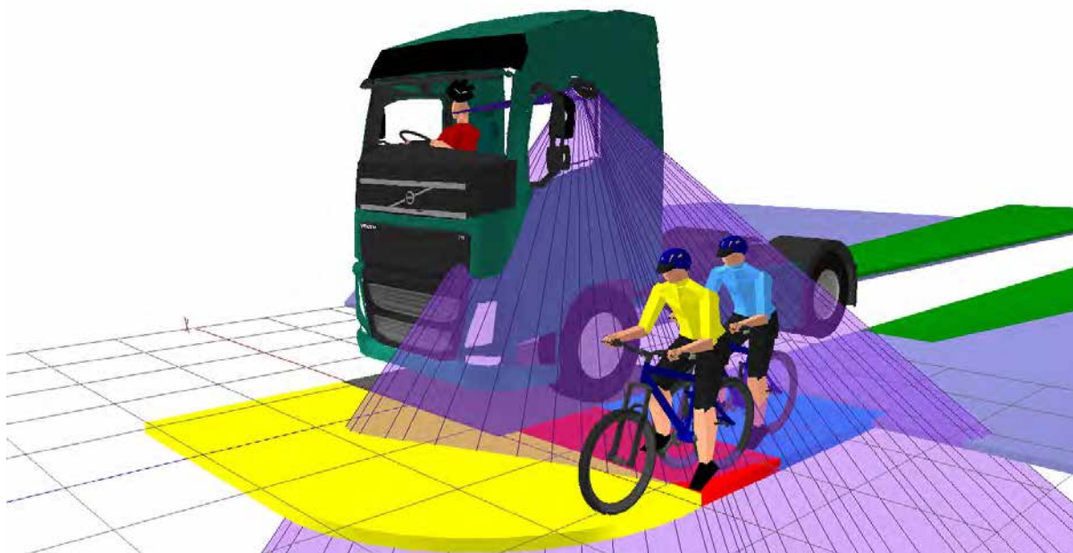
Figure 753. 3D volumetric projection showing the visibility of cyclist VRUs to the nearside of a vehicle with a 5 th %ile UK female driver using the Class V mirror adjusted for a 95 th %ile UK male
