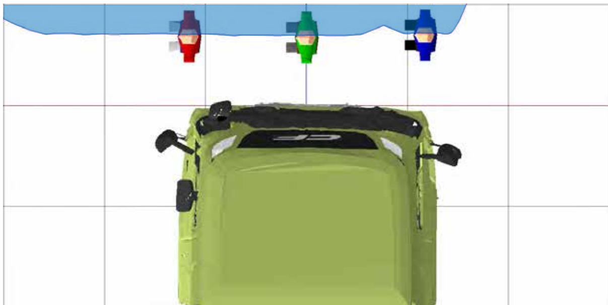
Figure 88. A plan view of the three human models that represent a pedestrian walking in front of a stationary vehicle and the projection of the windscreen at a height that equals the stature of a 50th%ile UK male pedestrian
