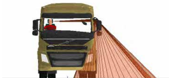
Figure 530. A front view of the Class V mirror projection for the Volvo FM N3
