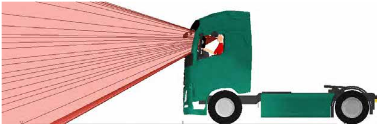
Figure 591. A side view of the windscreen aperture projection for the Volvo FH N3
