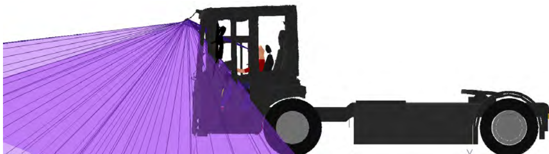
Figure 369. A side view of the Class VI mirror projection for the Mercedes Econic LEC
