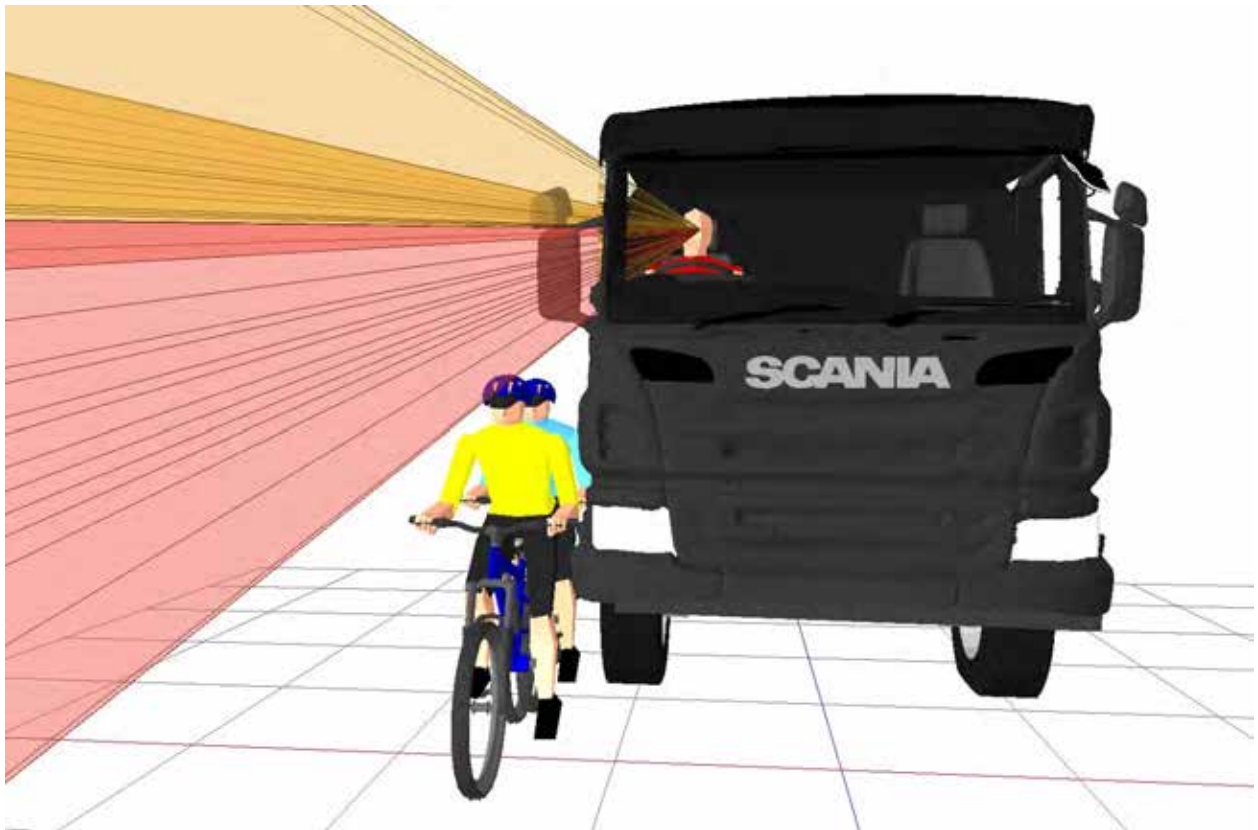
Figure 446. 3D view showing that front (yellow) cyclists cannot be hidden from direct vision and the rear (blue) cyclist can be just hidden from direct vision to the offside of the Scania P N3G
