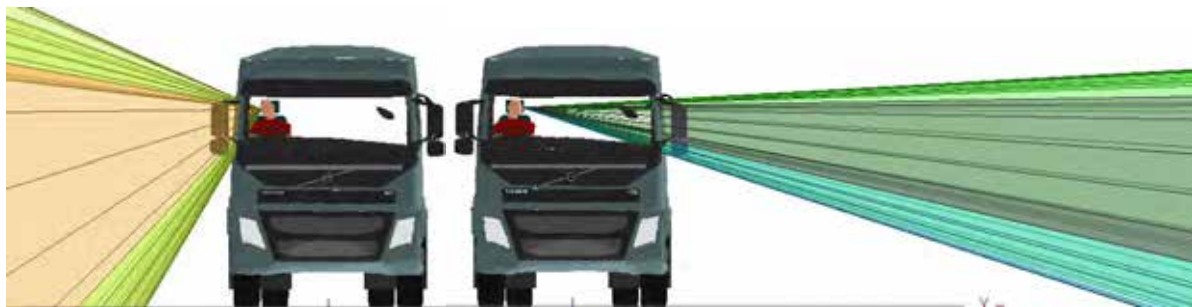
Figure 560. Frontal views of the off side and near side door window projections for the Volvo FMX N3G
