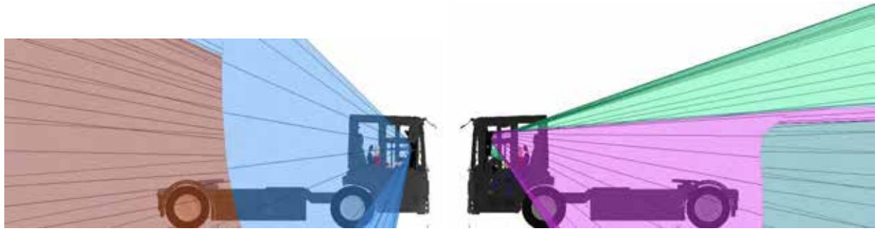
Figure 371. Side views of the combined Class II and Class IV mirror projections for the Mercedes Econic LEC
