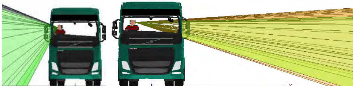
Figure 592. Frontal views of the off side and near side door window projections for the Volvo FH N3
