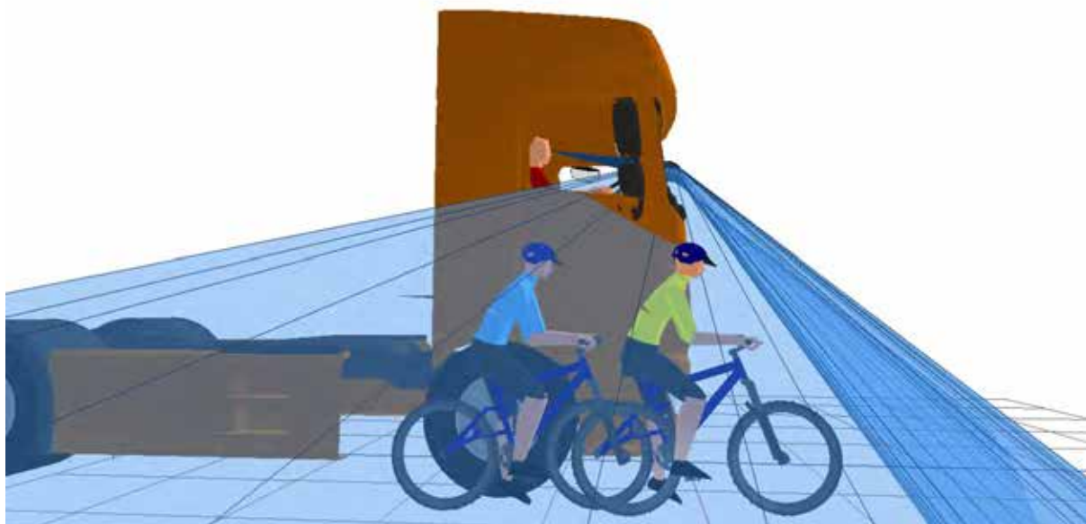
Figure 130. 3D view showing that the front (yellow) cyclist positioned to the offside of the vehicle is visible in the projection of the Class VI
