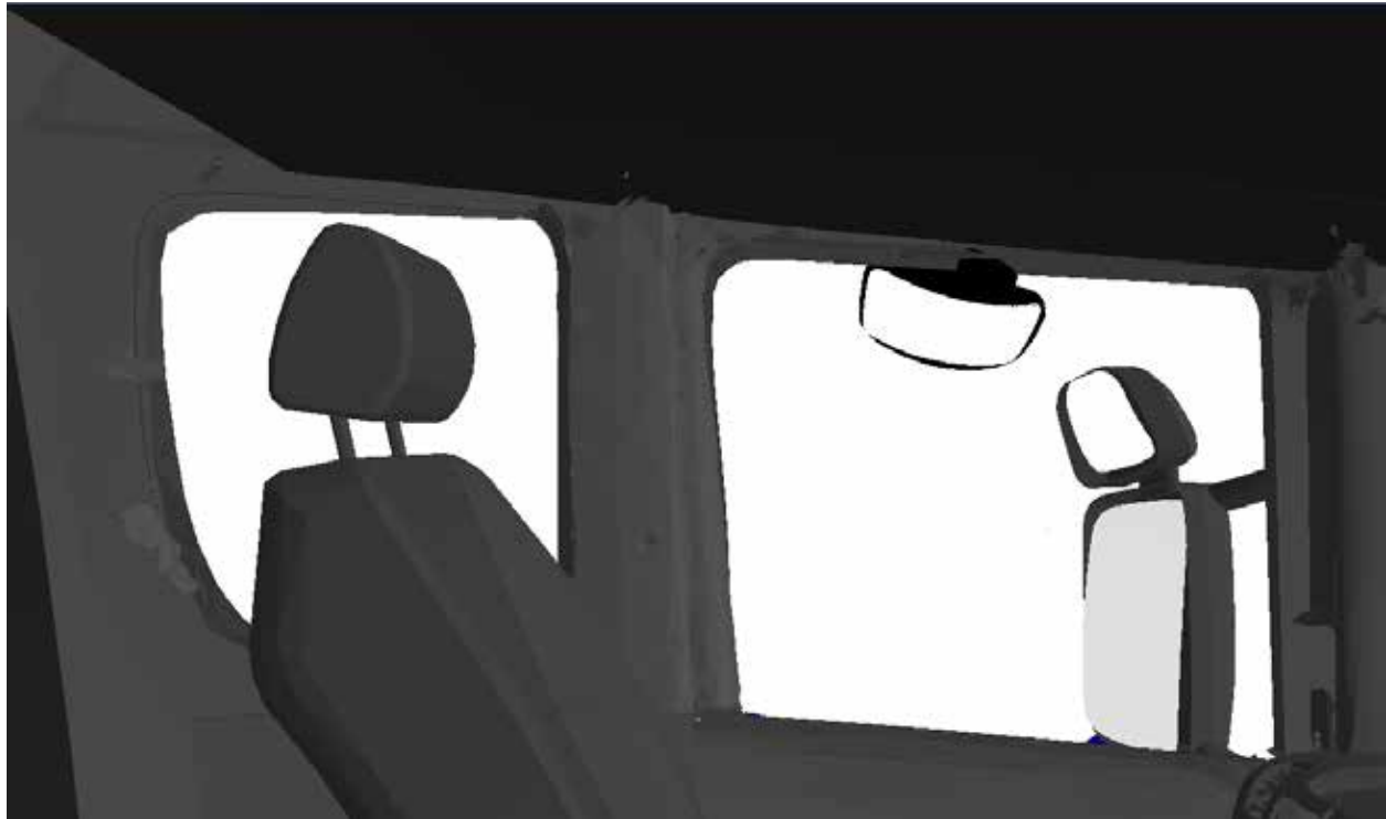
Figure 486. The view from the driver's eyes clearly shows the two cyclists are hidden from view.
