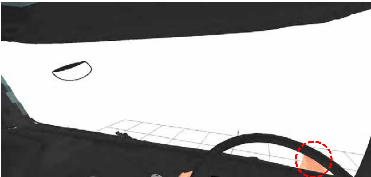
Figure 569. The view from the driver's eyes shows that all three pedestrians are hidden from view, though the right (blue) pedestrian may be visible through the centre of the steering wheel depending on its design.
