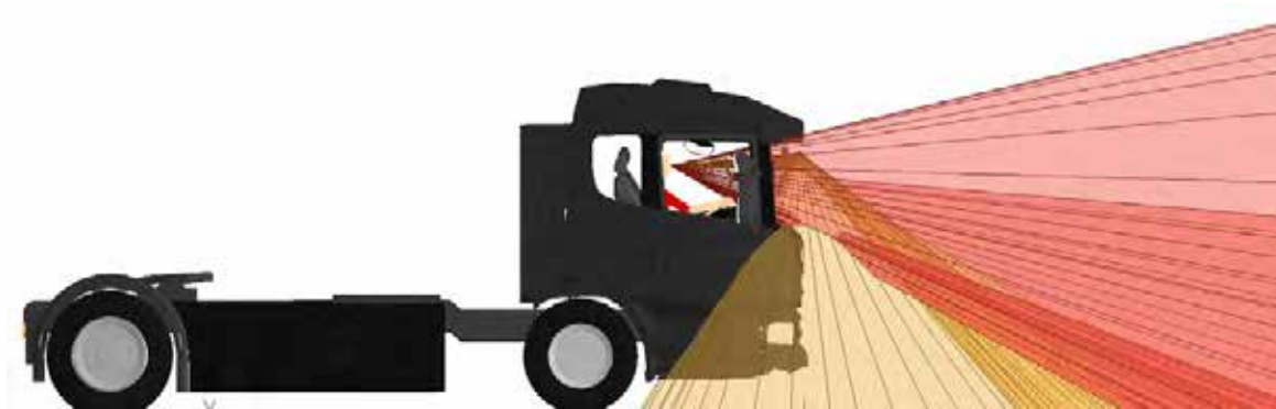
Figure 500. Combined projection of the windscreen and Class VI mirror to the front of the Scania N3 LEC
