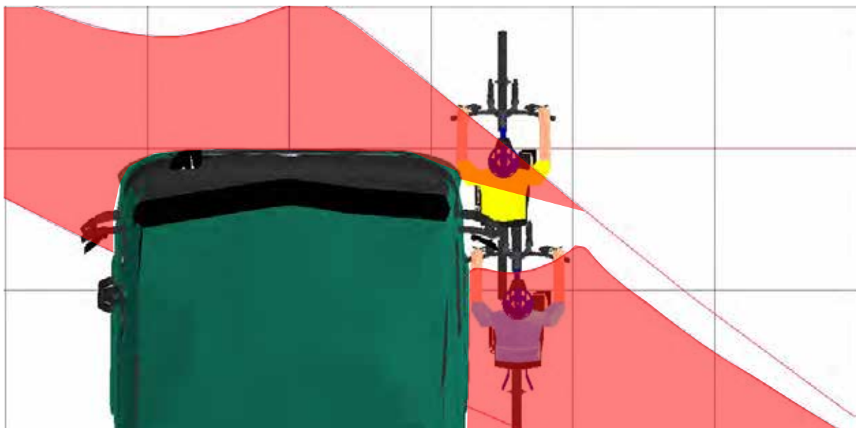
Figure 609. A plan view of the two human models that represent a cyclist moving past on the outside of the vehicle and the projection of the Class IV and Class VI mirrors at a height that equals the stature of a 50th%ile UK male cyclist
