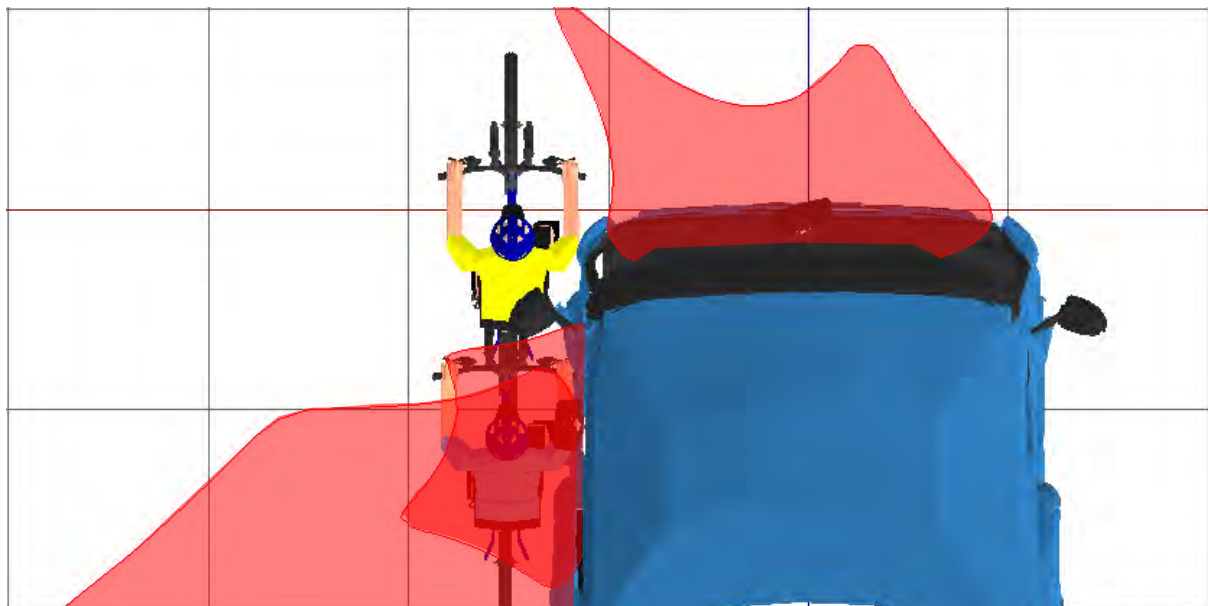
Figure 648. A plan view of the two human models that represent a cyclist moving up the inside of the vehicle and the projection of the Class IV, Class V and Class VI mirrors at a height that equals the stature of a 50th percentile UK male cyclist
