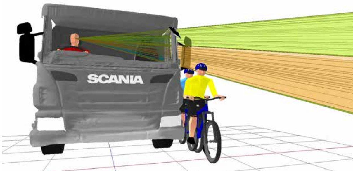
Figure 421. 3D view showing that the two human models can be seen through direct vision by the driver in the standardised driving posture
