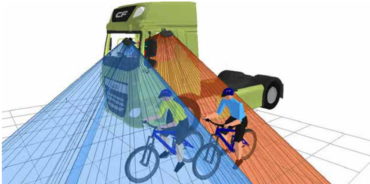
Figure 105. 3D view showing that both cyclists positioned to the nearside of the vehicle are visible in the projection of the Class V and / or Class VI mirrors
