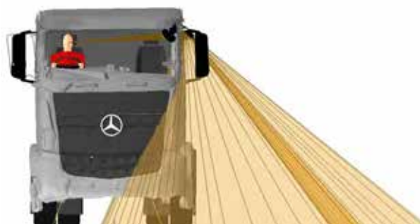
Figure 338. A front view of the Class V mirror projection for the Mercedes Actros N3
