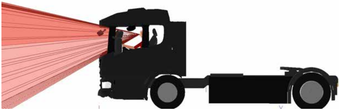
Figure 495. A side view of the windscreen aperture projection for the Scania N3 LEC
