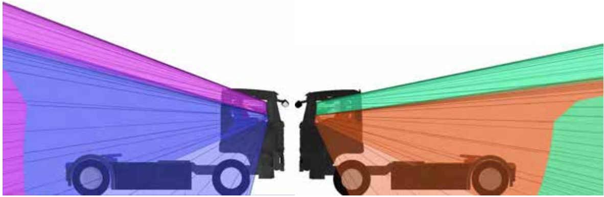
Figure 212. Side views of the combined Class II and Class IV mirror projections for the MAN TGS N3G
