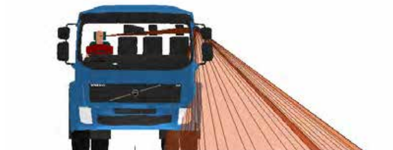
Figure 627. A front view of the Class V mirror projection for the Volvo FE N3 LEC
