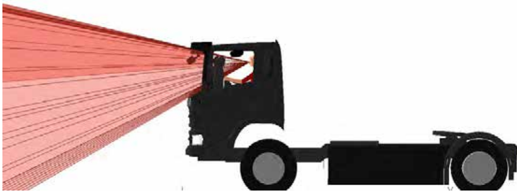
Figure 431. A side view of the windscreen aperture projection for the Scania P N3G
