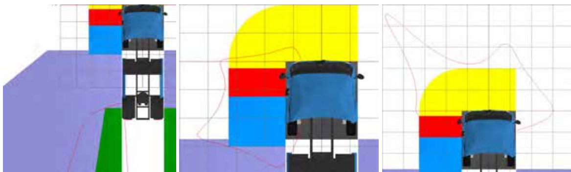
Figure 14. Example of mirrors (coverage outlined in red) adjusted to mandated areas for the Volvo FE LEC: Class II (left), Class V (middle), Class VI (right).
