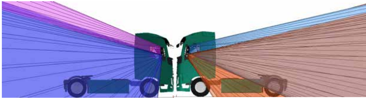
Figure 595. Side views of the combined Class II and Class IV mirror projections for the Volvo FH N3
