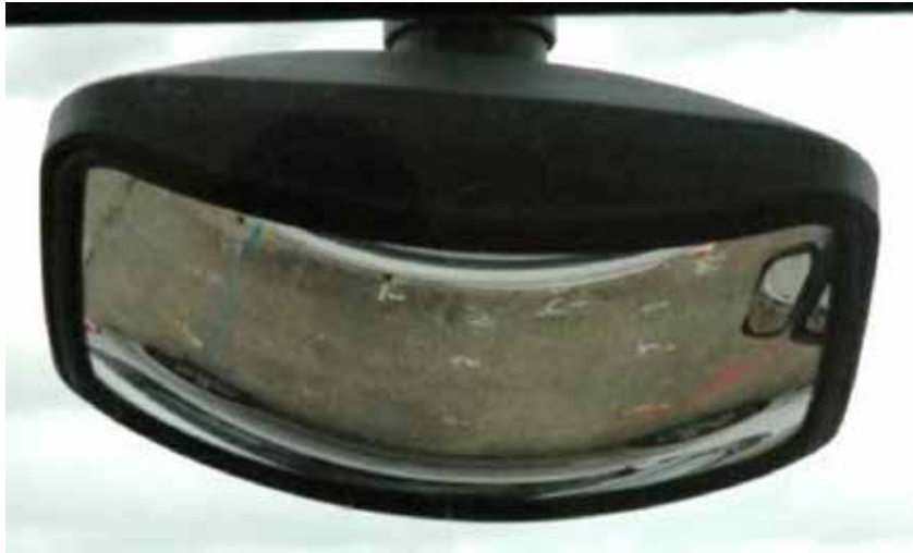
Figure 730. The view that a driver has of a Class V 'Look Down' mirror showing a silver car adjacent to the cab
