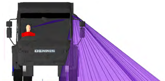
Figure 147. A front view of the Class V mirror projection for the Dennis Eagle Elite 6 LEC
