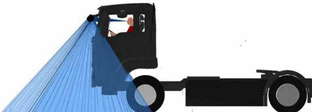
Figure 210. A side view of the Class VI mirror projection for the MAN TGS N3G
