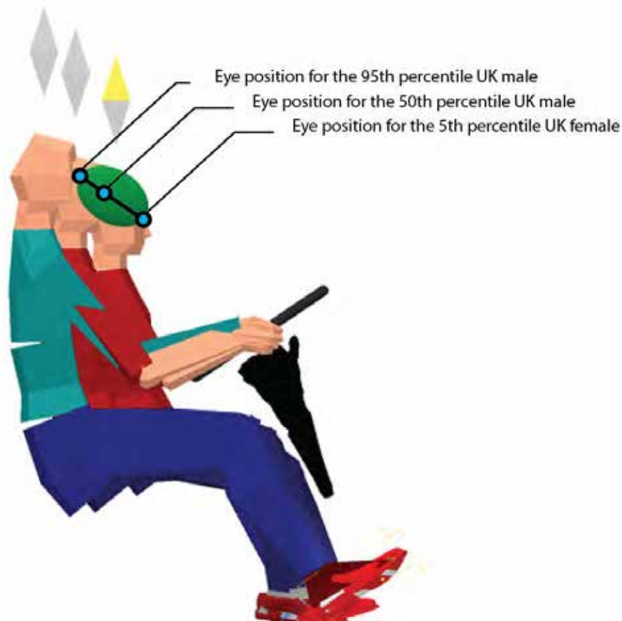
Figure 8. An example of the postures that were defined by the location of the Eyellipse and the available adjustability of the seat and steering wheel
