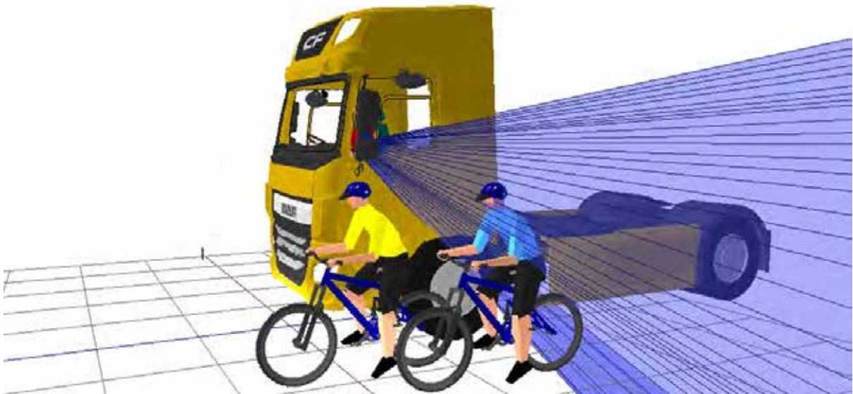
Figure 74. 3D view showing that the rear (blue) cyclist positioned to the nearside of the vehicle is visible in the projection of the Class IV mirror
