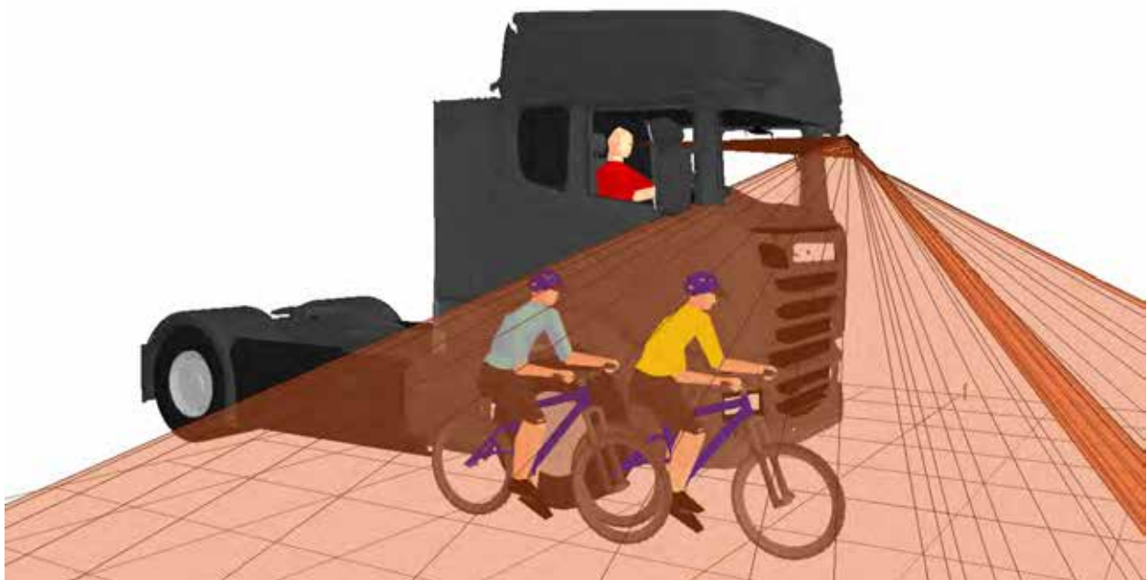
Figure 481. 3D view showing that the front (yellow) cyclist positioned to the offside of the vehicle is visible in the projection of the Class VI
