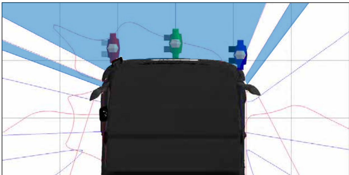
Figure 503. A plan view of the three human models that represent a pedestrian walking in front of a stationary vehicle and the projection of the windscreen at a height that equals the stature of a 50th%ile UK male pedestrian
