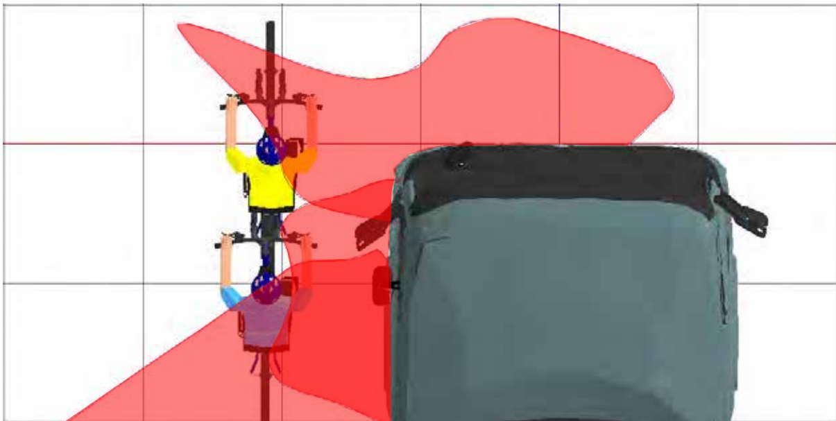
Figure 583. A plan view of the two human models that represent a cyclist moving up the inside of the vehicle and the projection of the Class IV, Class V and Class VI mirrors at a height that equals the stature of a 50th%ile UK male cyclist
