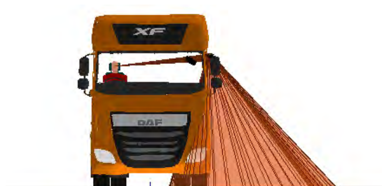
Figure 115. A front view of the Class V mirror projection for the DAF XF N3
