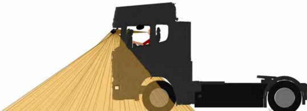
Figure 465. A side view of the Class VI mirror projection for the Scania R N3
