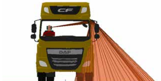
Figure 51. A front view of the Class V mirror projection for the DAF CF N3
