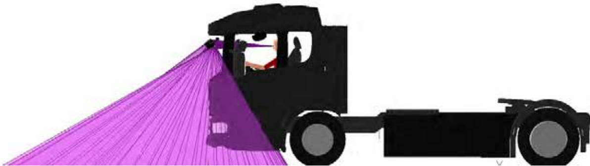
Figure 497. A side view of the Class VI mirror projection for the Scania N3 LEC
