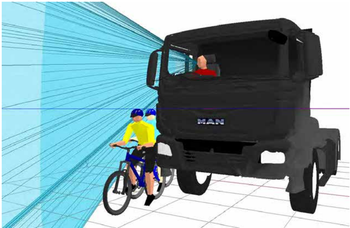
Figure 223. 3D view showing that both cyclists can be hidden from direct vision to the offside of the MAN TGS N3G
