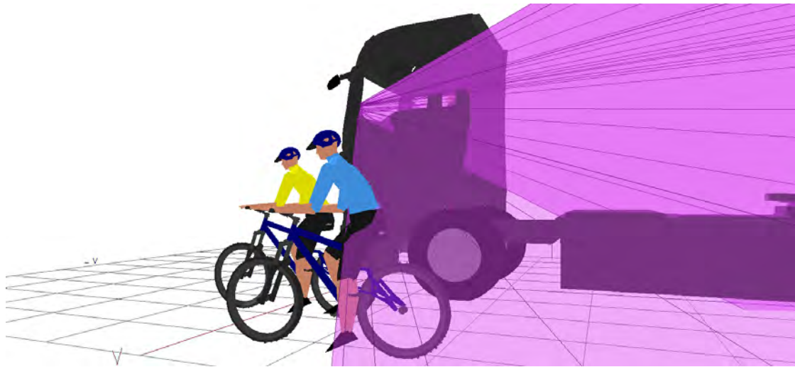
Figure 265. 3D view showing that the rear (blue) cyclist positioned to the nearside of the vehicle is visible in the projection of the Class IV mirror
