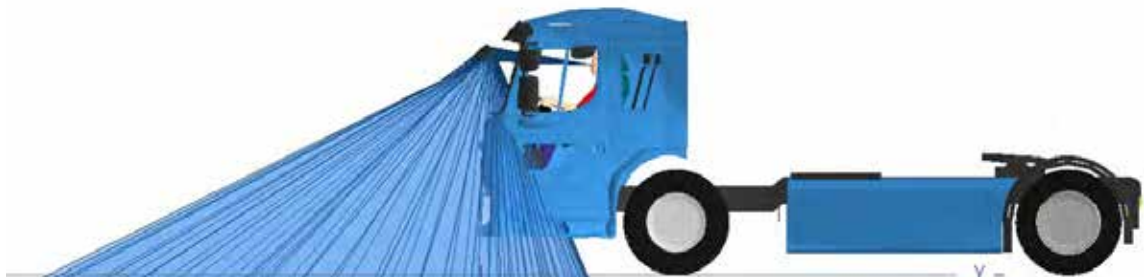
Figure 626. A side view of the Class VI mirror projection for the Volvo FE N3 LEC
