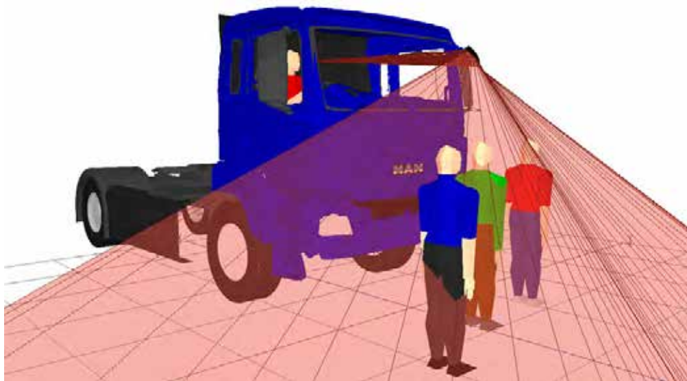
Figure 188. 3D view showing that all three pedestrians positioned to the front of the vehicle are visible in the projection of the Class VI mirror
