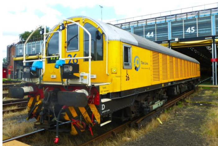
Figure 3: Battery Locomotive at Ruislip Depot
