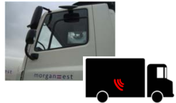
Fresnel lens Beeping motion sensor
