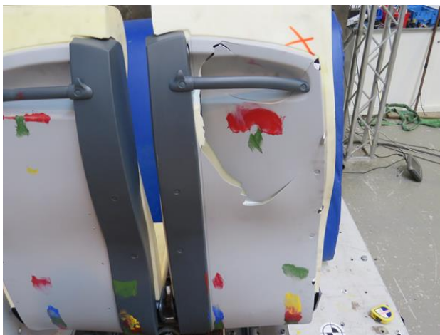
High backed seat: failure (splitting) of rear panel in area where dummy head impacted
