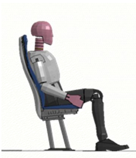
Figure 5-10: 50 th percentile Hybrid III dummy sat in bus seat with ‘high back’ showing that seat back is not high enough to support head fully if occupant propelled into their own seat
