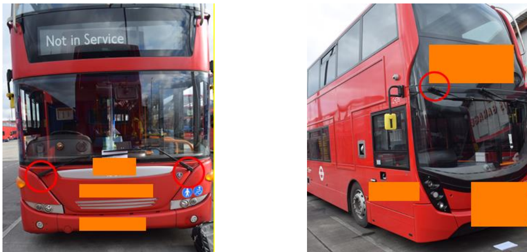
Figure 2-41: Protruding wiper driver posts positioned in pedestrian impact zone (left) and above pedestrian impact zone (right)
