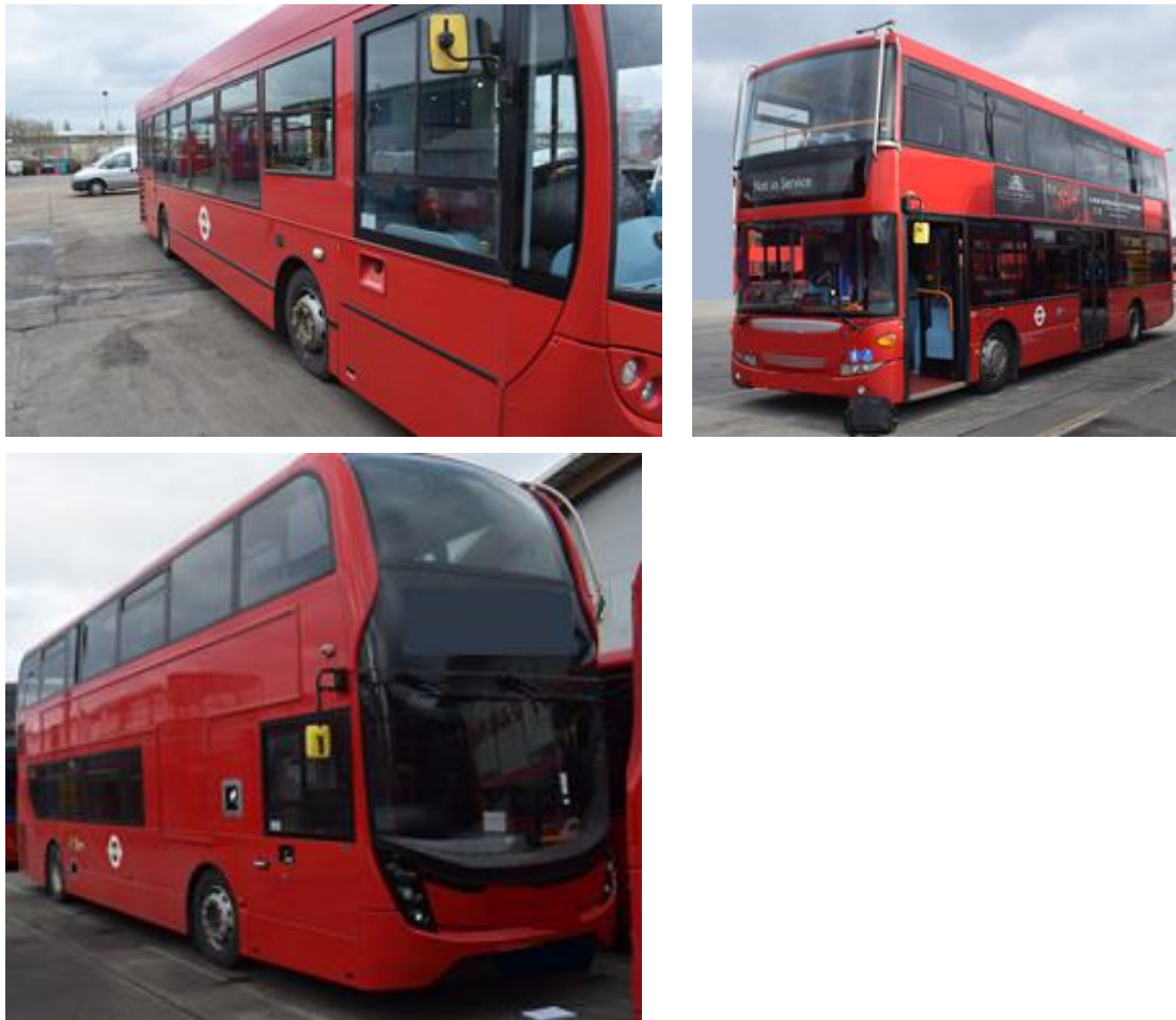
Figure 2-40: Views of bus exterior showing generally flat surfaces with no significant protrusions with the exception of mirrors and wiper driver posts on some buses
