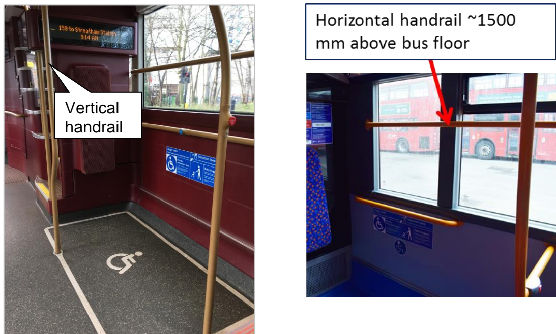
Figure 2-27: Vertical and horizontal handrails in head impact zone in wheelchair area
