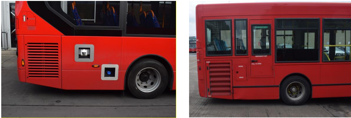
Figure 2-42: Filler points recessed (left) and covered with hinged flap (right)
