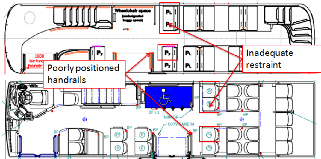
Figure 2-34: Poorly positioned handrails and inadequate restraint for seats behind middle doors and wheelchair area
