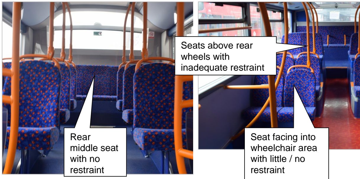
Figure 2-32: Little / no restraint of passengers on middle seat on back row (left) or seat facing into wheelchair area (right). Also, inadequate restraint for higher seats (above rear wheels) with inadequate restraint from low backed seats ahead of them
