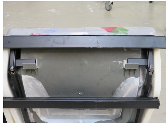
Low backed seat: failure causing detachment from pedestal legs
