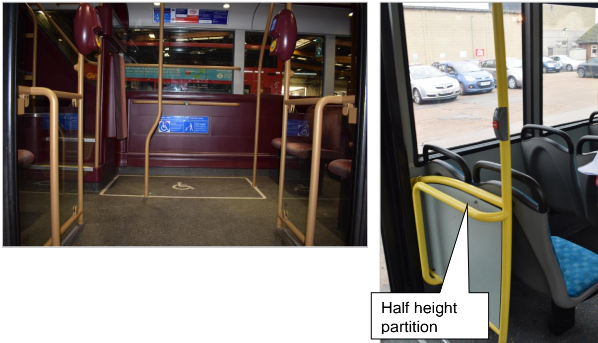
Figure 2-28: Half height partition to left of middle doors
