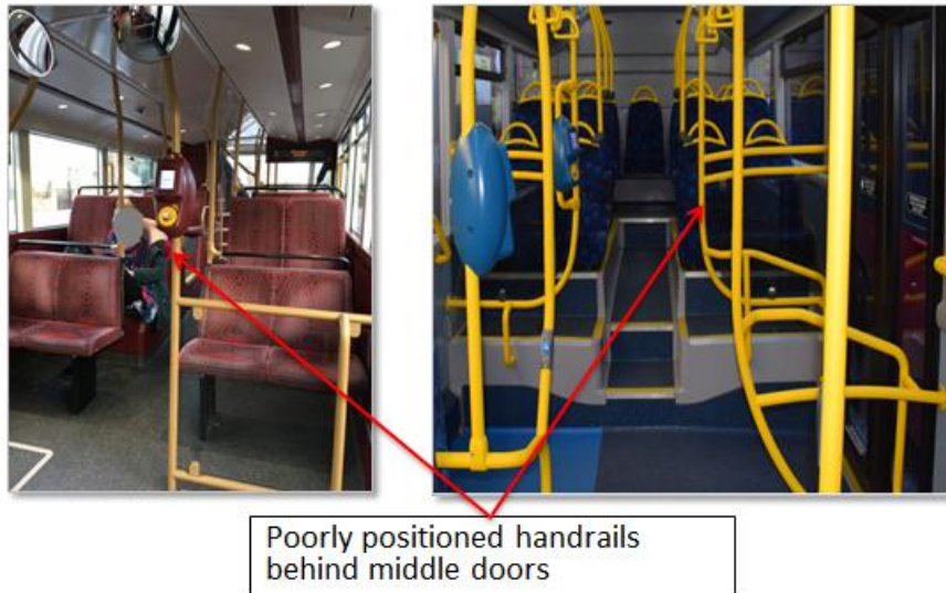
Figure 2-36: Poorly positioned handrails for seats behind middle doors
