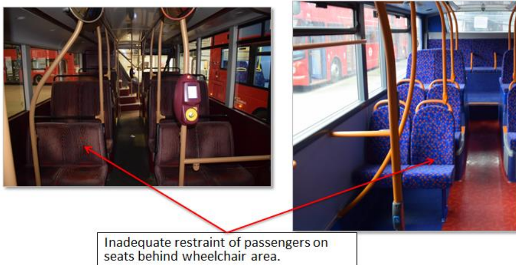
Figure 2-35: Inadequate restraint of passengers on seats behind wheelchair area
