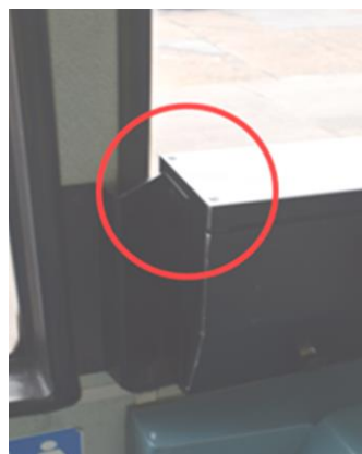
Figure 2-33: Sharp corners on passenger information display by priority seats
