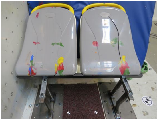
Low backed seat: splitting of rear panel in area where dummy legs impacted
