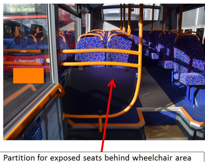
Figure 2-37: Example of partition installed to improve passenger restraint for exposed seats behind wheelchair area
