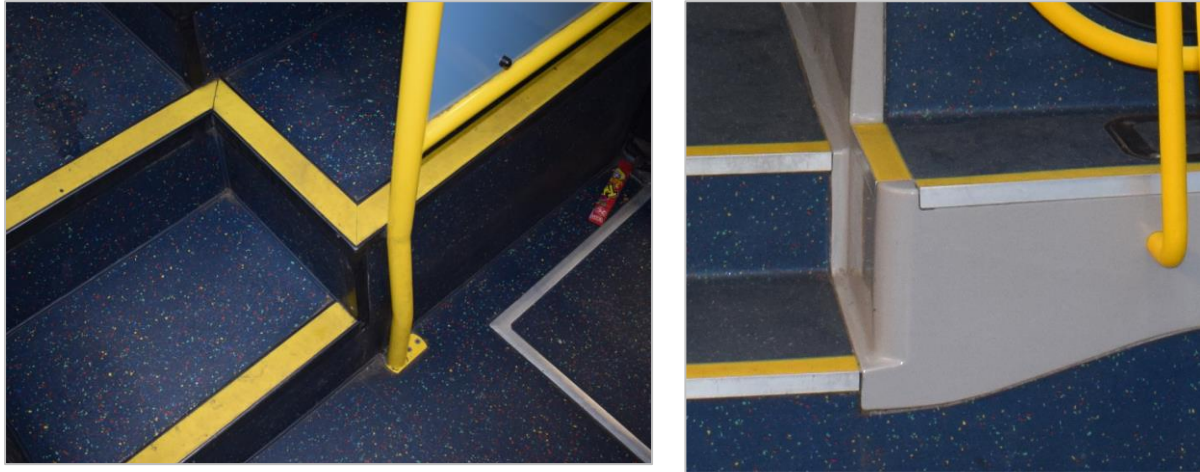
Figure 2-29: Sharp step corner (left); rounded step corner (right)
