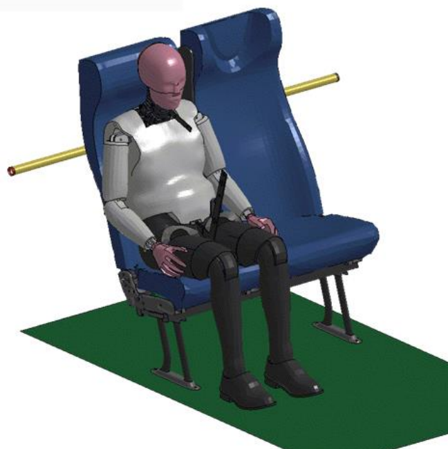
Figure 5-26: Iso view of BioRID II dummy in high backed (coach) seat with modified head restraint foam (recess filled in) to improve support for head rearward motion
