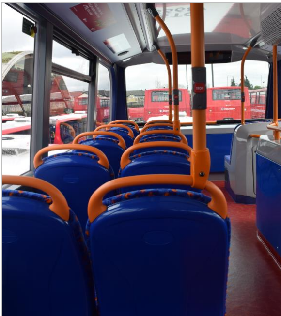
Figure 2-31: Example of low backed seat, handrail on top can be impacted by passenger seated behind (left) and if rear facing provides no support for head/neck of passenger (right)
