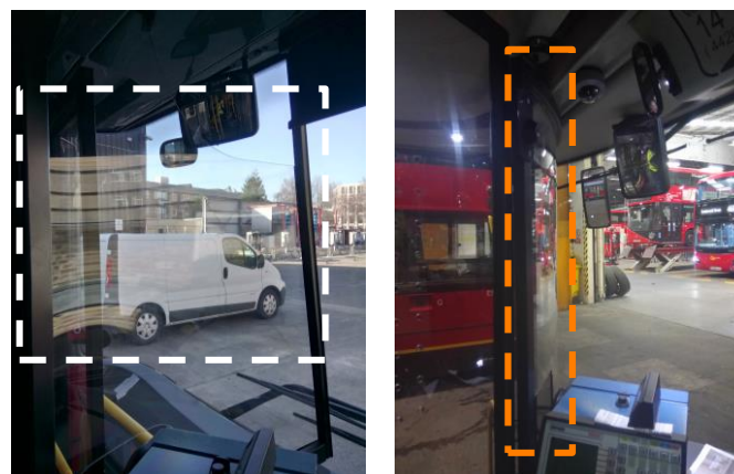
Figure 39: Partial A-pillar overlap and reflectance through a Curved Inwards DAS (left). Unobstructed view of external and internal mirrors and area of optical distortion and reflectance caused by Curved Away DAS (right)
