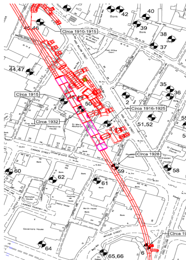
Figure 1 - Borehole Location Impacted by Tunnel Alignment
