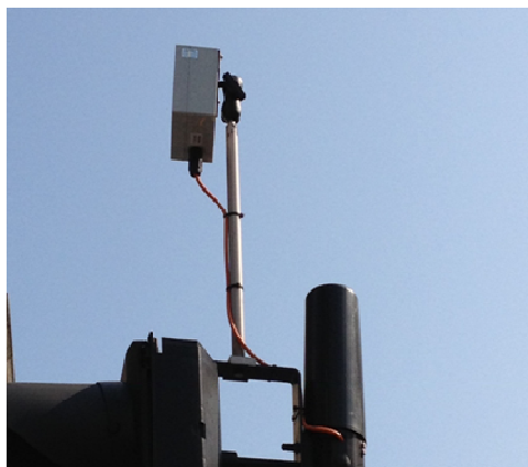
Access point which receives the vehicle, detected from the in-road magnetometer
