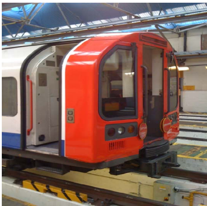
'92 tube stock cab end replacement in progress
