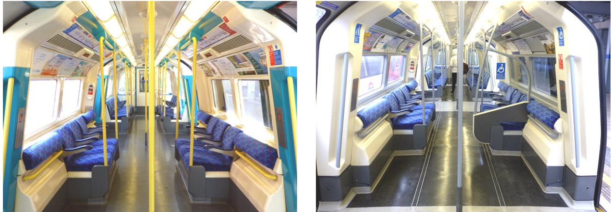
Figure 3: Jubilee line new wheelchair bays and refurbishment, before and after
