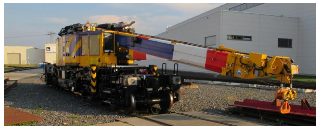
Figure 9: Mod P&C Kirow Crane
