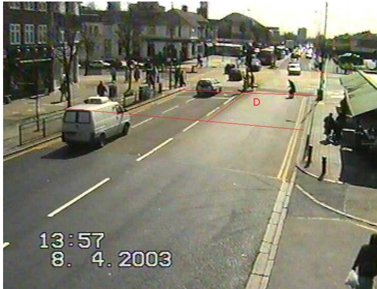
Figure 5.1: Reference Lines used for Speed Measurement
