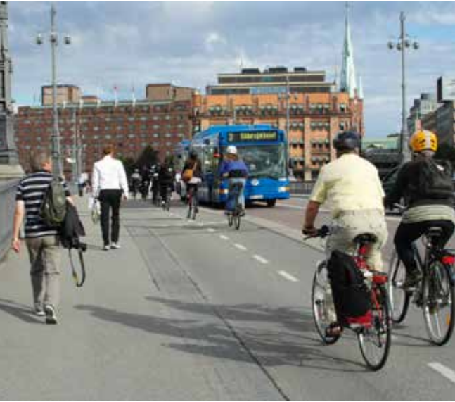
A bi-directional cycle track on a bridge, created by re-assigning a general traffic lane
