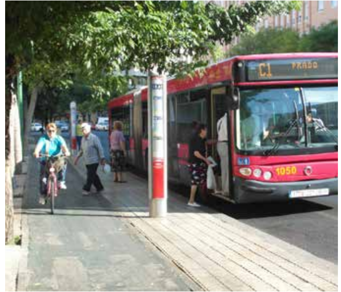
A typical 'floating bus stop' arrangement.
