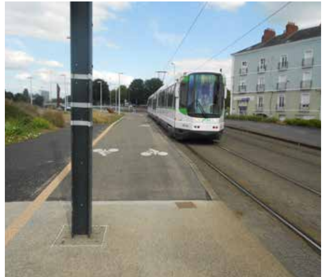
New bi-directional track running parallel to a tram line
