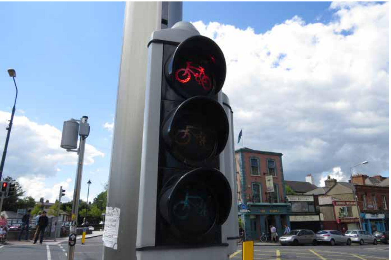
Ireland has been using low level cycle signals for many years
