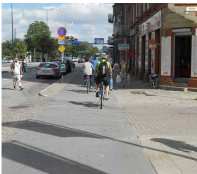
Cycling through Malmö's inner suburbs en route to Lund - protected bi-directional track with priority over side roads
