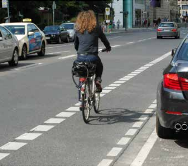
Typical cycle lane layout - with 0.5m 'dooring zone' allowance
