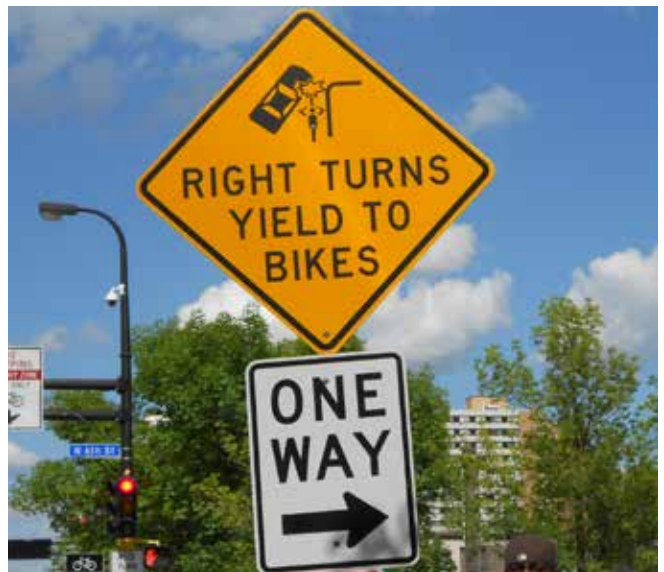
Sign apparently erected in response to a 'right hook' problem
