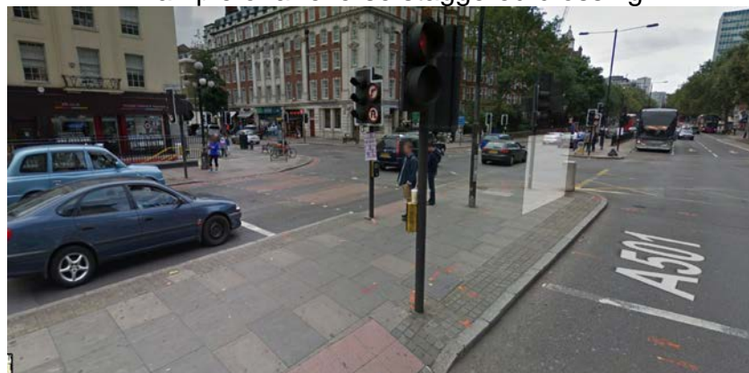
Example of a reverse staggered crossing
