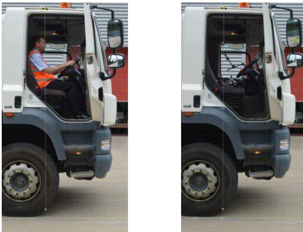
Figure 6: Comparison of the driver seating and eye position and the position of the steering wheel mounted laser assessment tool (DAF Tipper)
