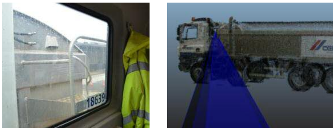
Figure 25: A photograph of the view through the rear window of the DAF Tipper and the visibility zone through the window shown on the model
