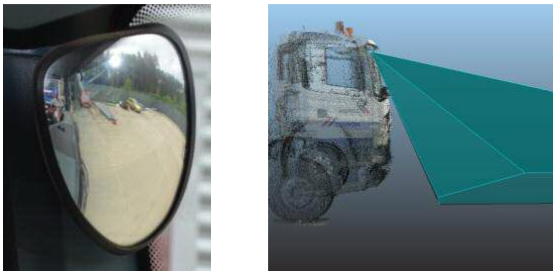
Figure 18: A photograph of the forward projection mirror fitted internally in the DAF Mixer showing that the front of the vehicle is not visible. The model shows the effect of the mirror being fitted rearwards of the front of the cab
