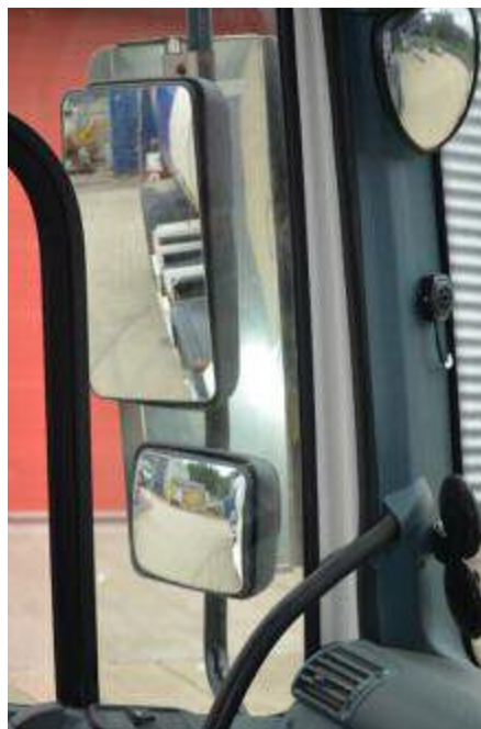
Figure 20: The position of the nearside side mirrors and the obstruction caused by them and the metal protective cover
