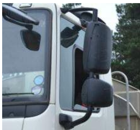
Figure 26: The photograph shows the gap between the plain rear view mirror (top) and the wide angle rear view mirror (bottom) on the DAF Tipper
