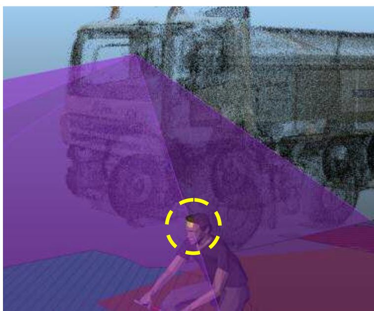
Figure 40: The 1.5m tall cyclist in position 9 showing the small area of forehead that is potentially visible in the lower nearside corner of the windscreen of the DAF Tipper
