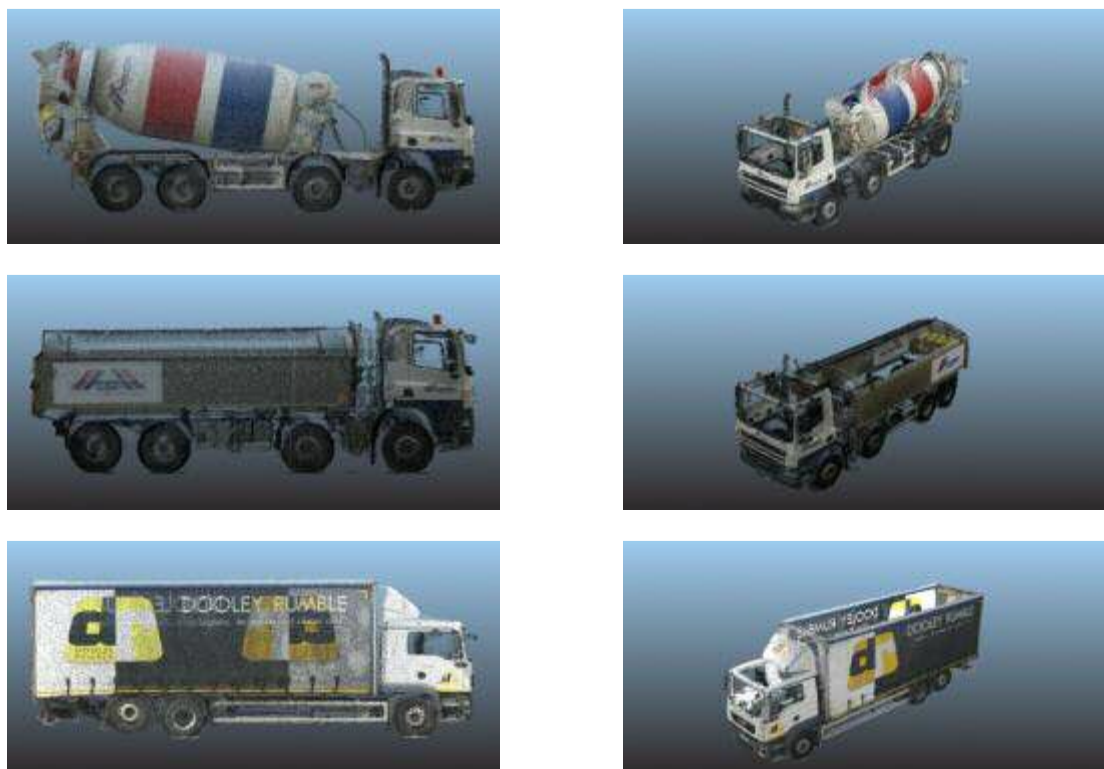
Figure 8: Point cloud images of the DAF Mixer, DAF Tipper and MAN Curtain side lorries
