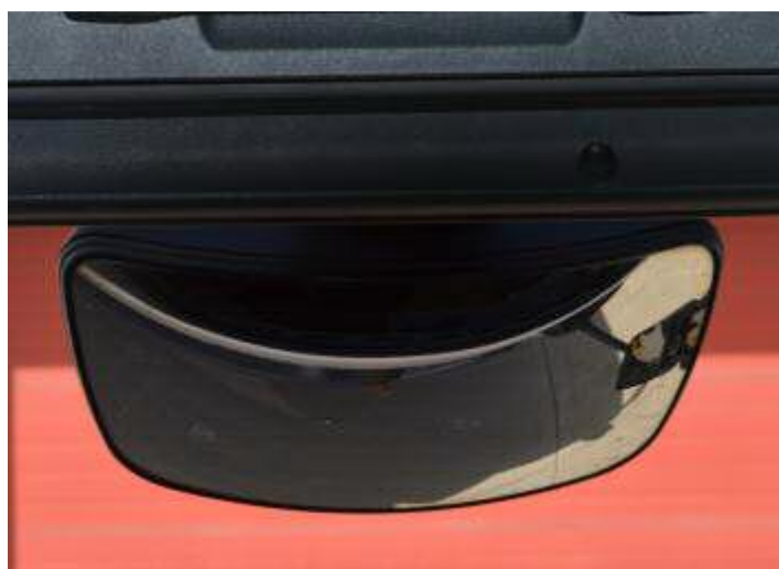
Figure 4: The Class V convex side close proximity mirror fitted to the MAN Curtain side lorry showing the distortion in the image to the straight line of the nearside side window frame where it appears curved in the image
