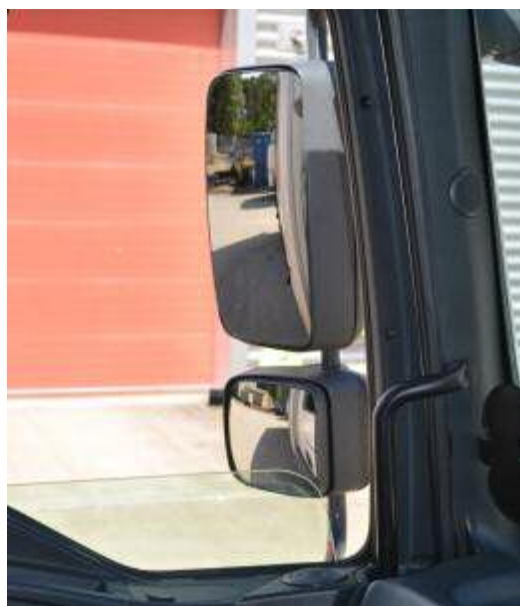
Figure 32: The nearside mirrors that were found to cause an obstruction to the view through the nearside side window of the MAN curtain side lorry
