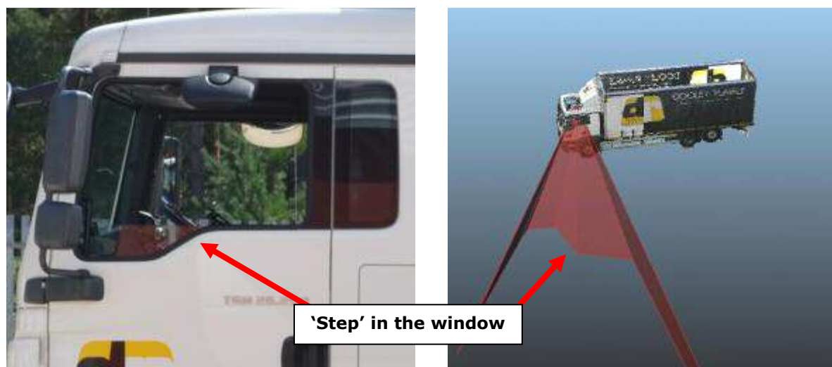
Figure 13: Image showing the effect of the 'step' shape in the window frame on the shape of the visible zone on the ground
