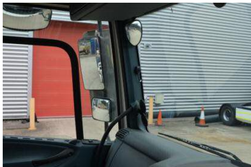
Figure 9: The direct view through the windscreen and side window for the DAF Mixer lorry and a photograph showing the A-pillar and mirror obstructions
