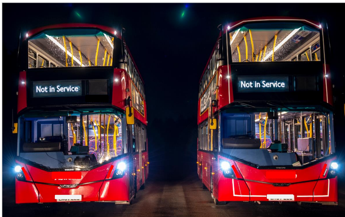
Figure 10: Test buses: Both buses are equipped with an additional pair of end-outline marker lights in the top corners (existing lights are just above the 'Not in Service' display); the bus on the right is additionally equipped with white reflective tape
