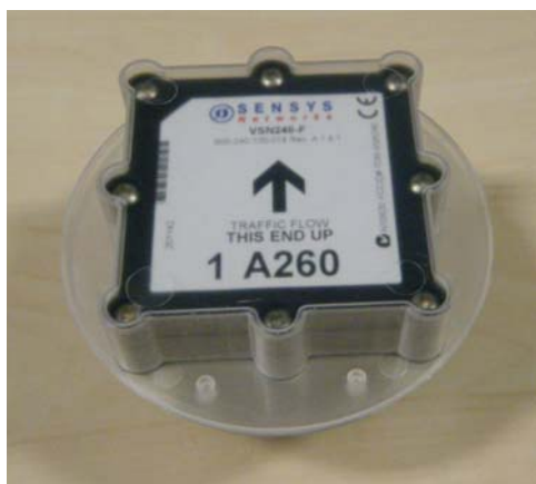
Magnetometer used as part of SCOOT installation
