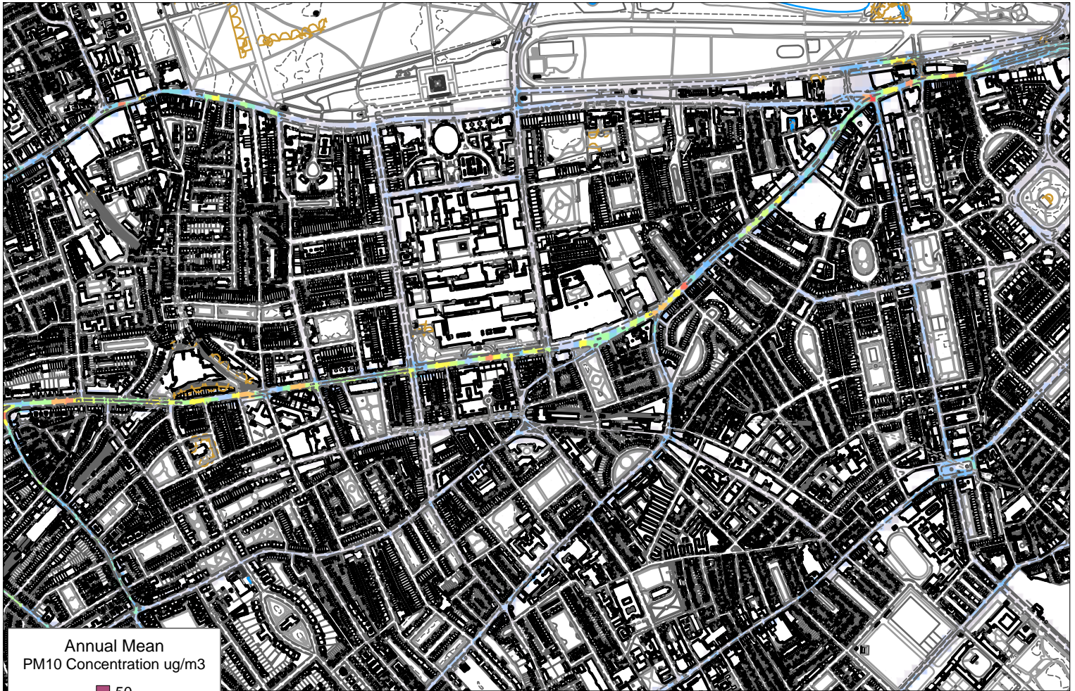
Predicted Annual Mean PM10 Concentrations in 2011 with WEZ Knightsbridge/Cromwell Rd/Thurloe Place/Old Brompton Road
