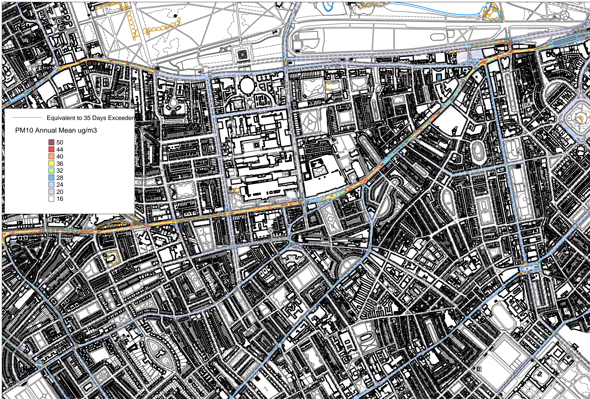
Predicted Annual Mean PM10 concentrations with contour representing 35 Exceedence Days of Daily PM10 with WEZ Removed (2011) Knightsbridge/Cromwell Rd/Thurloe Place/Old Brompton Road
