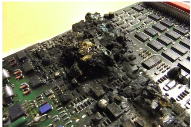
Propulsion system electronic card - damaged beyond repair
