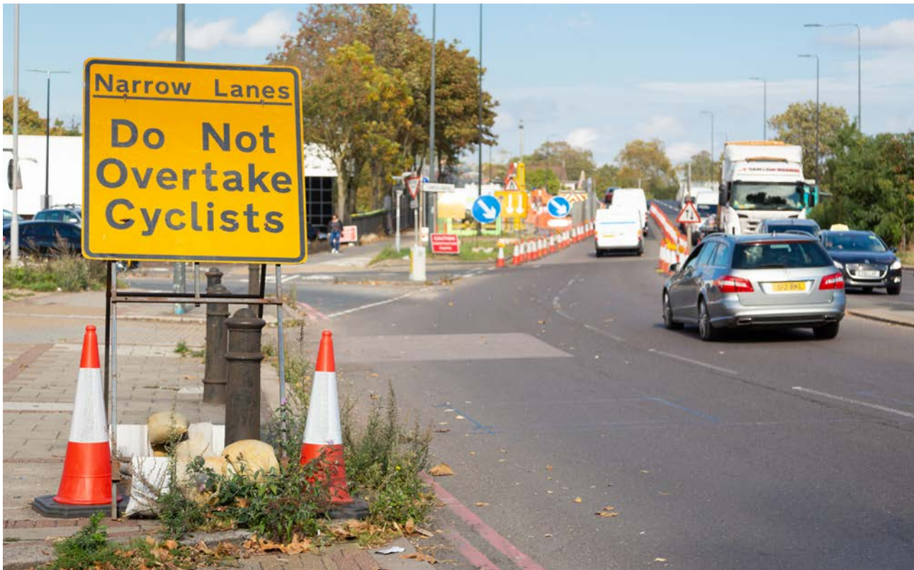
Warning sign should not be black and yellow
