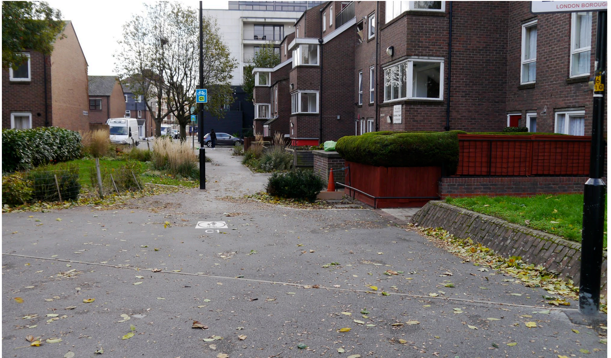
Housing land (LA), mid link – non-prescribed (use of off-highway inset markings and route confirmatory sign).
