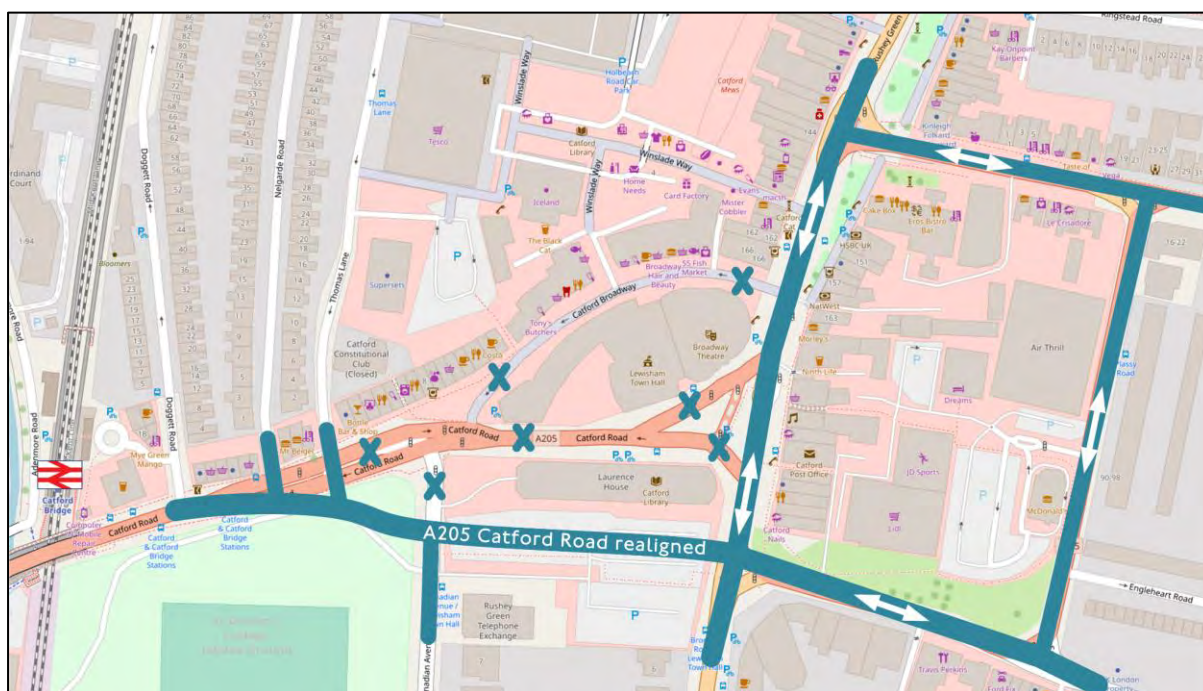
Figure 30 Schematic of proposed changes to the road alignments and gyratory system
