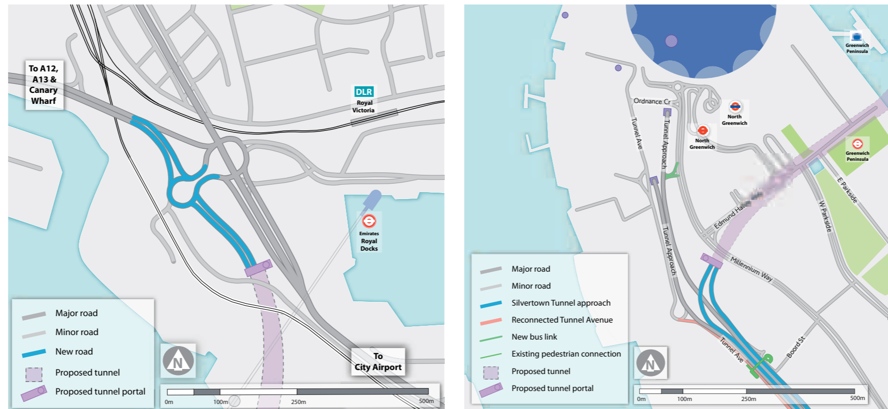
Figure 3.3 Map illustrating proposed connection of the Silvertown Tunnel to the existing road network, taken from the New East London River Crossings consultation document Oct 2012 - Feb 2013.
