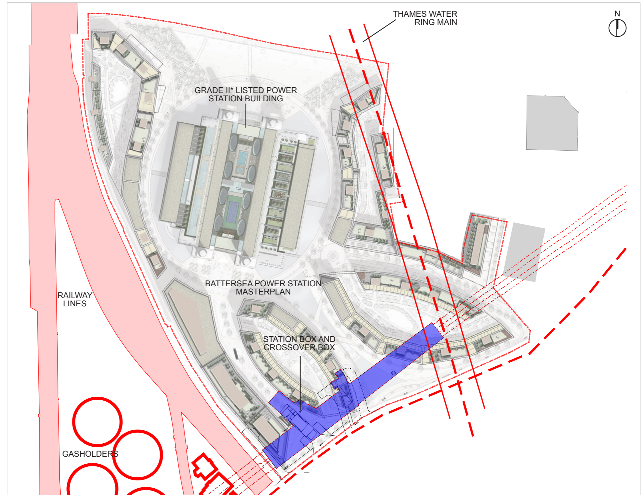
Figure 3.15 Battersea Station – Existing Site Constraints
