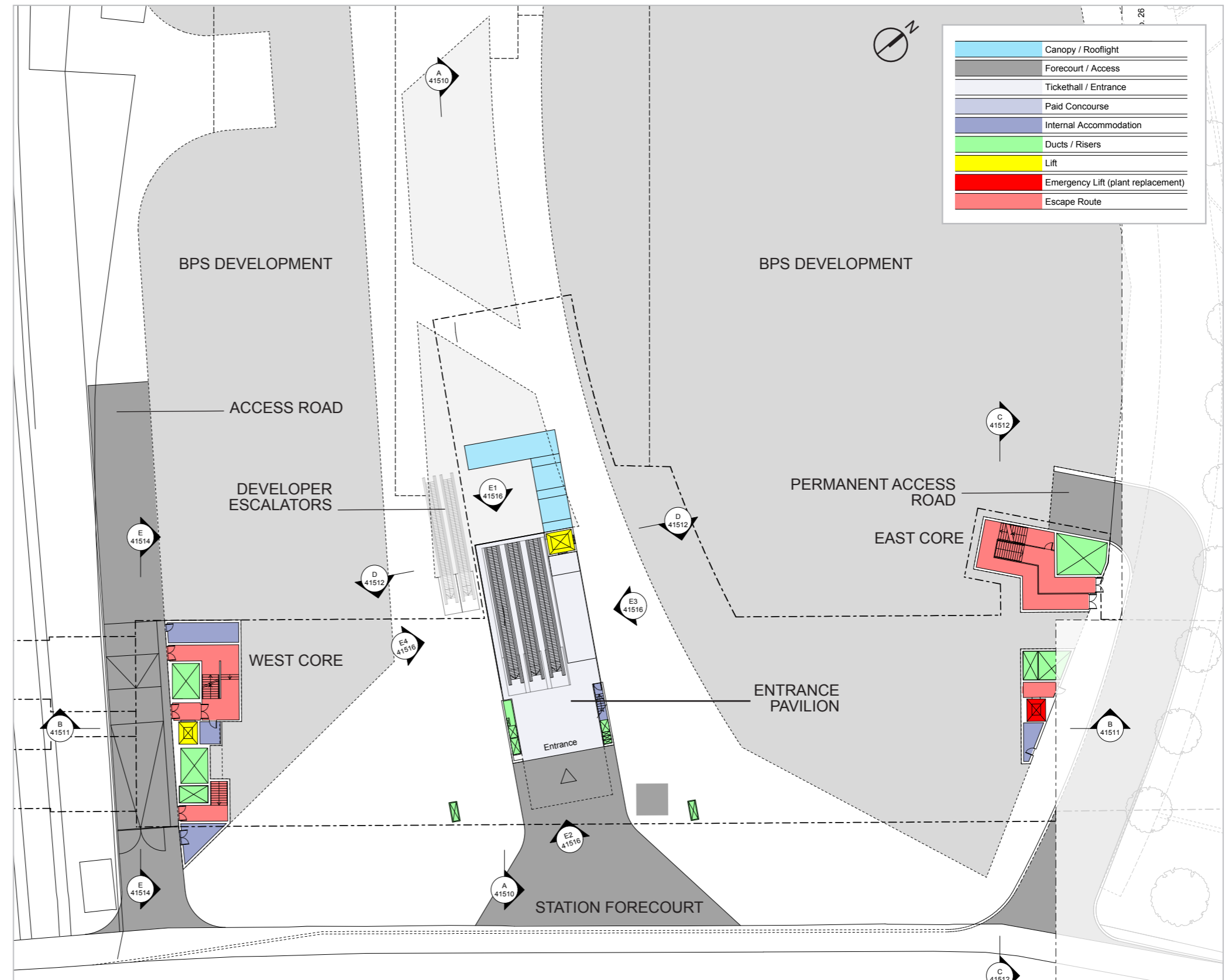
Figure 3.17 Battersea Station – General Arrangement Plan, Ground Level
