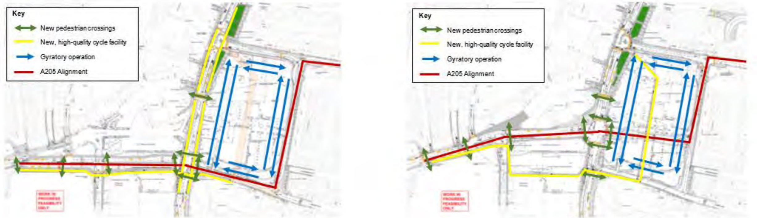
Figure 23. Design approach 3: Gyratory removal and A205 realignment (Realignment of A205, gyratory converted to two-way operation with substantial elements of work beyond highway boundary, active travel improvements)
