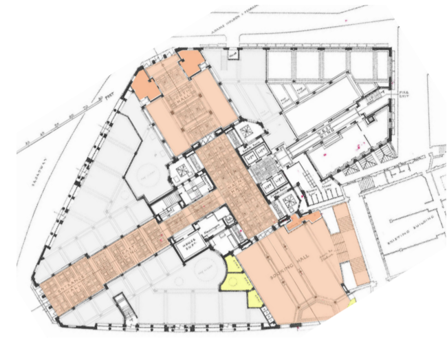
Original Holden plan illustrating the minimal retail and circulation route
