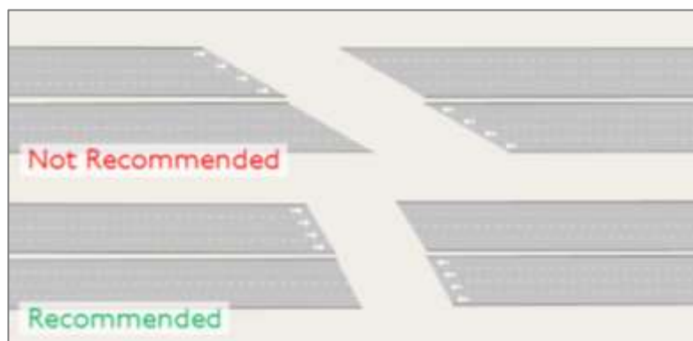
Figure 32: Angled Section entrances and exits. The top row would be considered too sharply angled.
