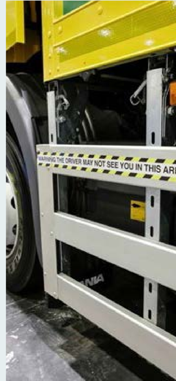
Side under-run protection must be fitted to both sides of the vehicle, unless demonstrably impractical
