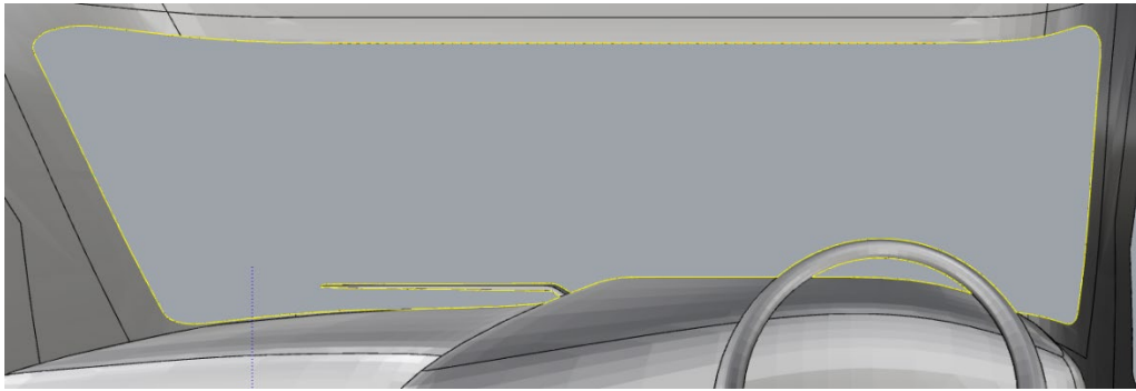
Figure 10. Creating the VOL (yellow path) for the windscreen, including the space between the steering wheel and the dashboard and accounting for the obscuration effect of the windscreen wiper
