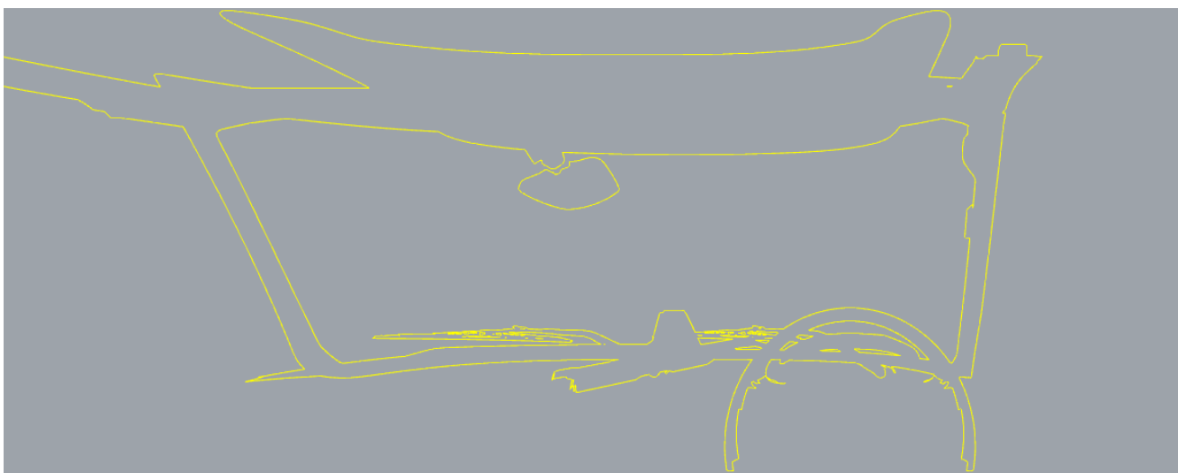
Figure 11. Outline of relevant geometry after use of the Rhino MeshOutline tool
