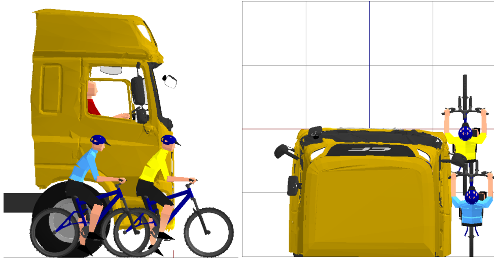
Figure 7. The direct field of view analysis to the right (driver side) of the vehicle highlighting the position of the cyclist models. The image to the left shows a side view of the vehicle. The image to the right shows a top-down view.
