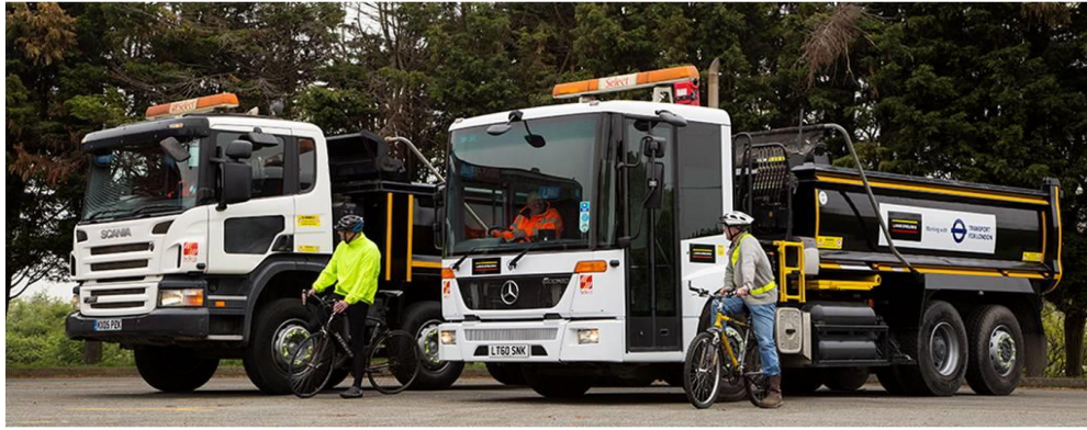
Figure 3: HGV construction cab compared to Mercedes Econic, five star HGV cab
