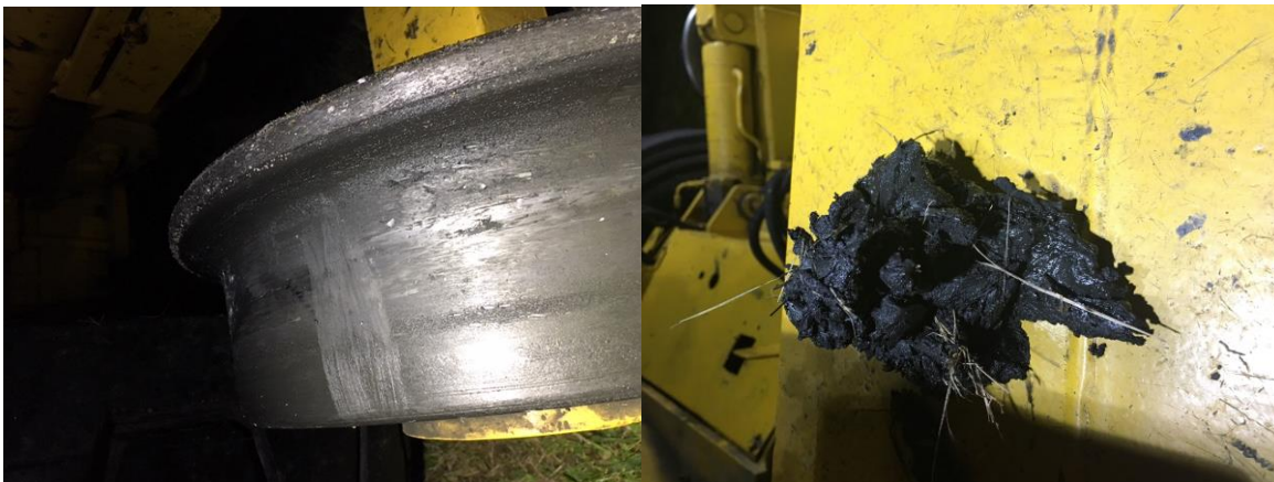
Image 1. Contaminated RRV wheel
