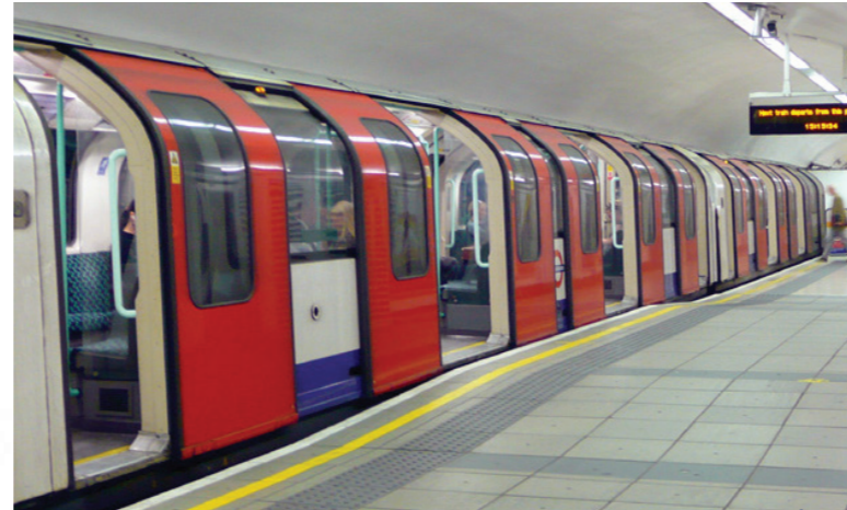
Figure 7.40: Example step-free access via platform hump
