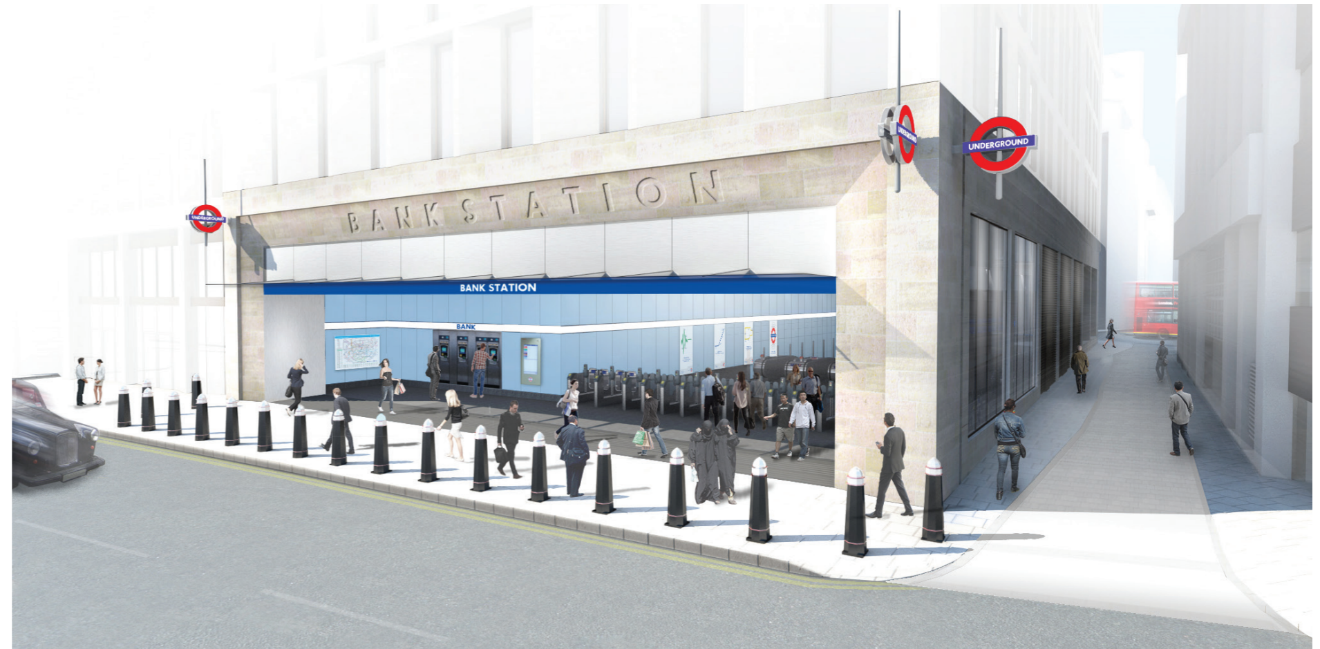
Figure 8.6 Visualisation of station entrance with functional LUL blue freeze, projecting canopy and 3D Roundels
