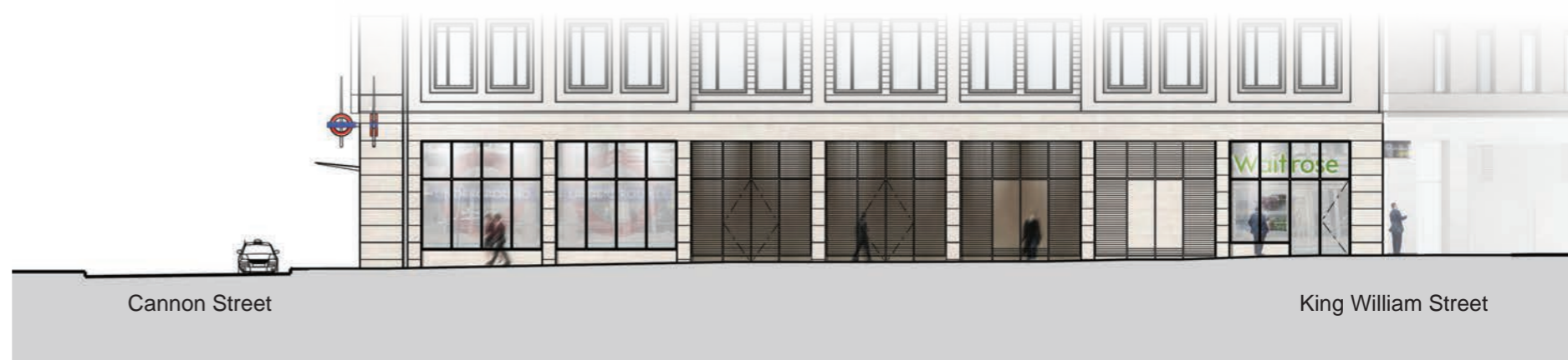
Figure 7.10: Contextual Nicholas Lane elevation of the new Station Entrance at ground level (OSD shown for information only)
